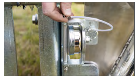
Pin adds security to the magnetic system
