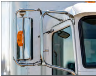
Marker light provides additional safety by signaling other drivers (select models)
