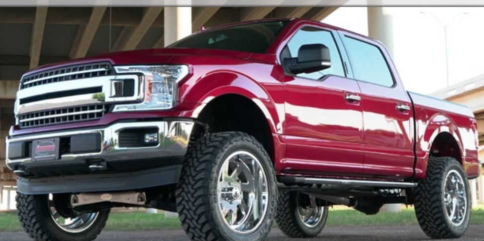
Rancho RS66506B with 35-in. tires. Trimming or modification may be required to provide proper tire clearance. Actual tire size varies between manufacturers. B designates black finish.
