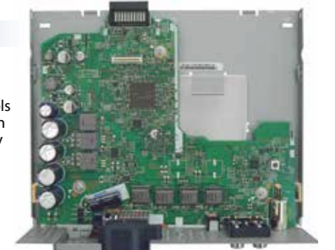
Large Capacitor and Plate-Type Heatsink
