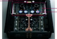
L/R symmetric circuit layout improves channel separation.
