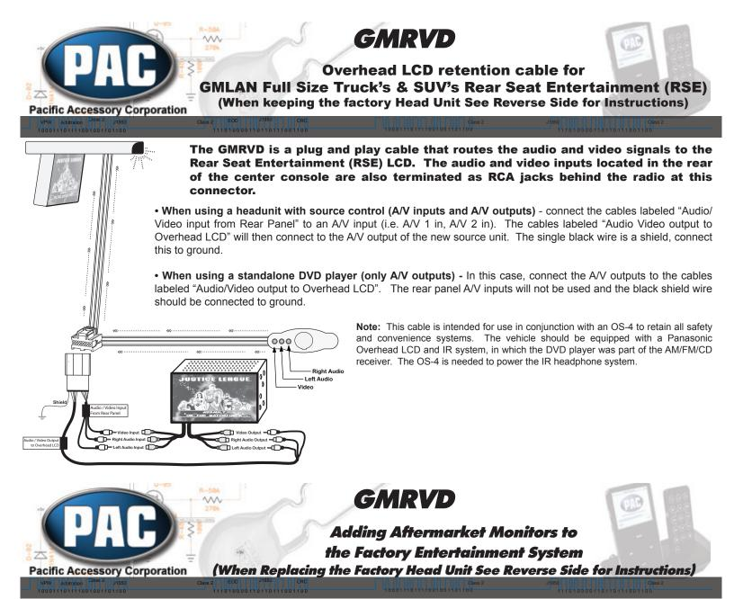
The GMRVD is a plug and play cable that allows aftermarket monitors and IR headphones to be connected to the factory entertainment system. The GMRVD is connected behind the factory head unit.
