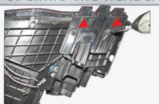
Start by using a phillips screwdriver to remove this bracket. There are 2 screws holding it in place.
