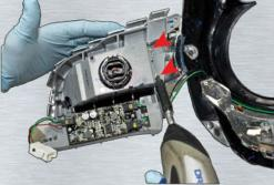
Loosen these 2 screw to seperate the reflector.
