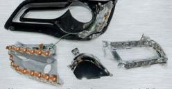
Here you can see that we have seperated all the main pieces of the headlight. Once this step is completed you can move onto the ribbon removal and install.
