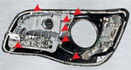
Here is an overview of the location of each screw needed to be removed.
