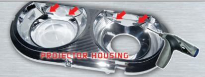
Drill four (4) slots into the top edge of the chrome housing. Each slot is for one edge of the halo to fit through. Notice the locations of where the slots are needed to be drilled. Allow yourself enough room for the edges of each halo to pass through the housing.
