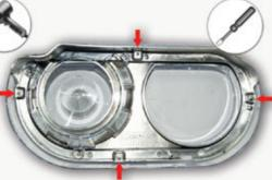
C) Remove the four (4) Phillips screws holding the chrome piece to the lens. The locations are marked with arrows.
