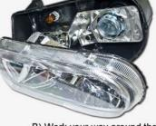
B) Work your way around the housing with a screwdriver. Prying through the sealant until the lens and the housing seperate. Take your time on this step.
