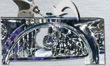
Again, drill another small hole into the chrome housing. Be precise with drilling. You do not want to scratch the chrome surface.
