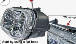
A) Start by using a flat-head screwdriver and apply pressure between the lens and housing. Caution, headlight will be hot.
