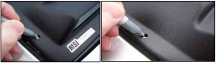
**Step 5.** Remove the masking tape and then carefully remove the RWL from the rear window glass and set aside on a clean surface, making sure that your marks on the glass are visible.
