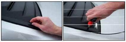
**Step 13.** With all the brackets now secure with a black nylon slotted nut, it is time to enjoy the ride...you have completed the installation.
