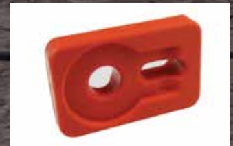
Winch Isolator PN: 1903931 Polyurethane isolator provides a clean and easy way to store the winch hook when not in use. Installed over the winch cable, the Winch Isolator nests with a roller and provides a convenient rest for the winch hook that also prevents it from rattling.
