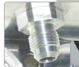
-6 AN inlet / outlet on pan
