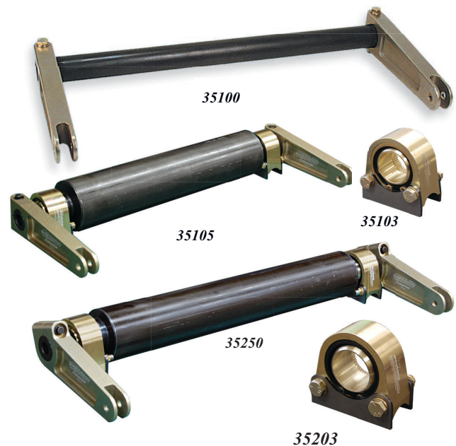
35250 3" Tubular Anti Roll Center Tube Assy 1-1/2" 3 X .083" X (24") center tube 35203 bearings (2), 1.5" ends, and 6" aluminum arms
