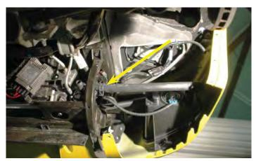
219. Cut 2" off the short end of the other supplied 3/4" x 4" x 36" elbow hose and connect to the passenger side barb on the heat exchanger using a supplied spring clamp. Route the long end of the hose through the same hole the driver side hose you just installed used.
