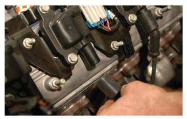
137. Unbolt the five bolts holding the coil brackets to the valve covers using a 10mm wrench.
