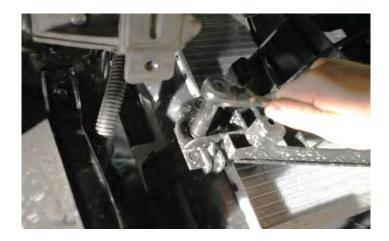
58. Remove the fan assembly by pushing up on the fan shroud to un-clip it from the radiator and then carefully pull the assembly out from the vehicle completely.
