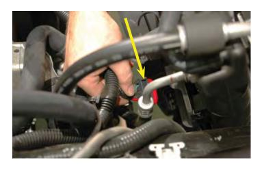
56. The fan shroud is held to the radiator by two bolts. One is located near the bottom of the radiator on the driver side. The other is located high on the passenger side. Use a 10mm wrench and remove this bolt.
