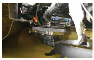
9. There are two computer connectors. Remove the connectors by first pulling the Red locking key out, then pushing in on the Black cover button and pulling the connector down.
