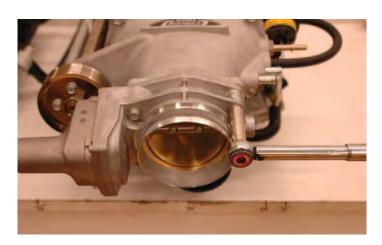
144. Remove the Manifold Absolute Pressure (MAP) sensor from the stock intake manifold using a Torx t-25 inverted socket. Ensure that the rubber seal is not missing or damaged as it and the sensor will be re-used.
