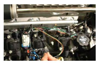
169. Re-tape the harness with the MAP sensor plug and wires removed to the junction of the wires near the center of the coil pack. After taping the remaining wires back up, tape the wires running to the MAP sensor plug as well.
