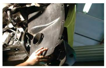
189. NOTE: For vehicles with brake cooling duct bolted to the inside of the fender well (as shown in this picture) follow the next two steps.
