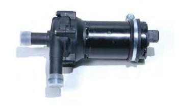
197. The pump will mount to the hole vacated by the push rivet you just removed. The discharge barb points to the passenger side fender, and the inlet toward the rear. The Adel clamp is at the end of the pump near the plug connection with the loop facing up and toward the passenger side fender. Tighten the supplied bolt and nut firmly.
