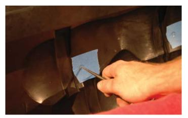
261. Use a 5/8" bit with an assistant holding a backing board behind the splash shield/air deflector to drill the two holes you just marked. You need to be careful, because a standard bit will bite through the plastic and pull the drill motor and bit into the heat exchanger close behind the splash shield. A Forstner bit or hole saw may work, but in any case, use extreme care to not damage the heat exchanger and radiator.
