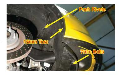
190. Use a 10mm wrench to remove the bolt at the inside surface of the fender well by the duct exiting port. Remove the push pin rivet on the front surface of the duct that connects the duct to the air inlet, and pull the brake cooling duct from the vehicle, set aside for later reinstallation.
