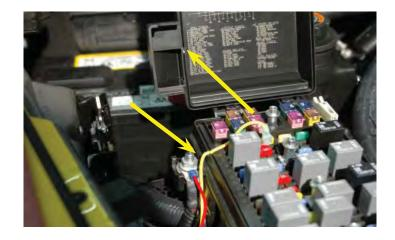
238. Use the provided self-tapping bolt to mount the relay of the harness to the sidewall by the existing fuse center as shown.
