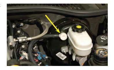
178. Route the hose forward along the coil pack, cut to fit and connect to the forward barb on the supercharger inlet.
