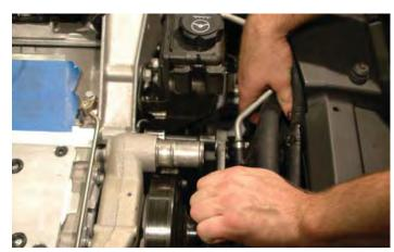
103. Remove the mounting bracket from the reservoir then remove the large hose from the bottom of the power steering reservoir by squeezing the clamp with a pair of pliers. Use a shop towel to catch any residual fluid. You may need to use a hook point to separate the hose from the barb as it may stick firmly in place.
