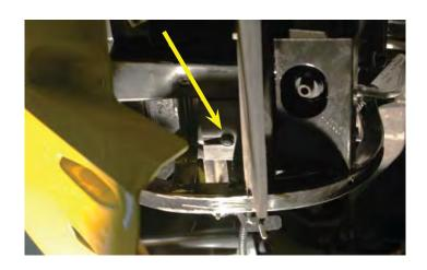
196. This is the intercooler coolant pump and its mounting clamp. Note: The plastic caps on the inlet and out should be removed before the hose connections are made.
