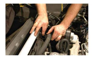
54. Use a small straight blade screwdriver to open the three harness clamps and release the wiring harness on the fan shroud.
