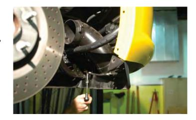
246. Attach the fender well splash shield, twisting to lock the brake cooling duct back into position and fasten using all the original hardware and locations. This includes push pin rivets and bolts.
