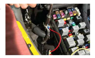
230. Zip tie the fuse holder to the hood release cable below the positive terminal of the fuse center as shown.
