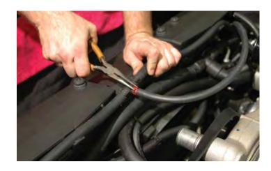
130. Loosely zip tie the hoses together, pass below the power steering reservoir and up toward the coolant vent pipe.
