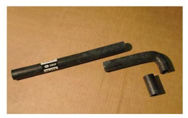
211. Install the supplied hose coupling (mender) in the long end of the remaining hose.
