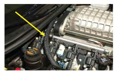
215. Remove the Adel clamp at the rear passenger side of the supercharger using a 10mm wrench.
