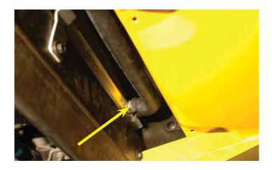
218. Route the hose through the holes you created in step #205, run over the turn signal enclosure and curve back to connect to the discharge barb on the intercooler pump as shown. Secure the hose with one of the supplied spring clamps.
