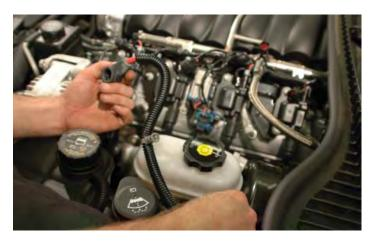
37. Remove the power brake check valve and hose from the brake booster grommet by pulling it out firmly.
