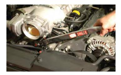
162. Install the new supplied supercharger and accessory fan belt with a 15mm tensioner wrench, using the new supplied belt routing diagram below.
