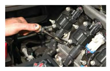
208. Install the supplied spacer between the valve cover and the rear bracket mounting hole of the intercooler reservoir assembly and replace the bolt back onto the valve cover from whence it came.
