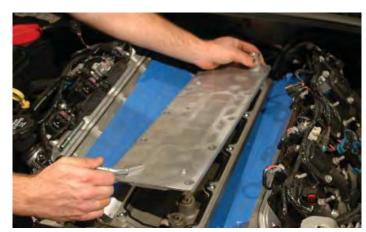
95. From the bottom of the original valley cover, remove the eight O-rings with a small straight blade screwdriver. Install the O-rings into the grooves in the bottom of the new valley cover.
