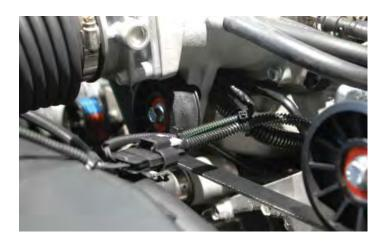
274. Replace the computer connectors in their original positions, making sure to lock them in place by pushing the grey levers towards the harness. Secure the connectors by inserting the red lock keys in position.
