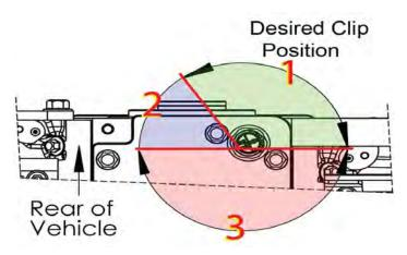
99. If the secondary locking clip lands in position #3, you will need to remove the sensor and re-clock it using the supplied copper shim. Before reinstalling, wrap the sensor's threads with Teflon tape or Teflon paste. Reinstall the sensor and shim into position #1 using a torque wrench to 15 ft-lbs minimum to 24 ft-lbs maximum.
