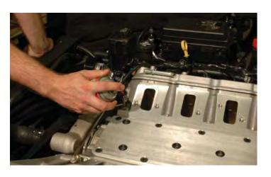
152. Carefully, set the supercharger assembly on the engine, line up the bolt holes with the holes in the cylinder heads. (Be careful of the one bolt located under the rear supercharger pulley on the passenger side as it protrudes and must be aligned first.)
