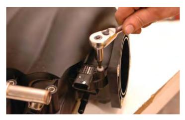
145. Apply a small amount of the grease supplied to the MAP sensor seal.
