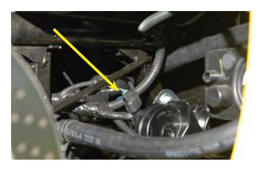
244. Inspect your coolant hoses carefully and add sections of the provided split loom to protect the hoses from any chaffing and rubbing on hard or sharp edges.
