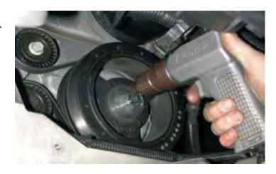
74. Using a 24mm socket, remove the large bolt and the drill guide from the engine.
