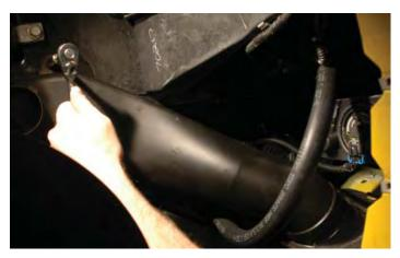
191. Squeeze the electrical connector to unplug the electrical connection from the horn assembly on the passenger side forward of the wheel well.
