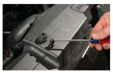
257. Insert two of the push pin rivets into the existing ¼" holes in the bottom of the new air-box standoff mounts. Push the "nails" back in locking the rivets in place.
