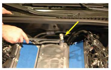
93. Use a 13mm socket wrench to remove the ten bolts that secure the engine valley cover.
