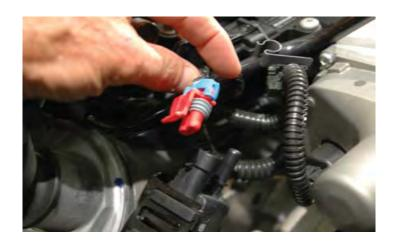
30. Disconnect the Electric Throttle Control (ETC) connector at the throttle body by squeezing the trigger connector and pulling to remove it.
