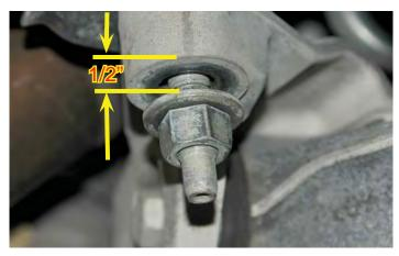
61. Remove the two motor mount nuts with an 18mm socket wrench.
