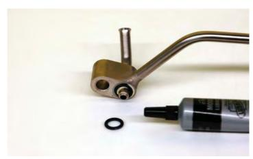
91. Install the new vent pipe with the original bolts and torque them with a torque wrench and 10mm socket to 106 in-lbs. Verify your torque wrench settings.
