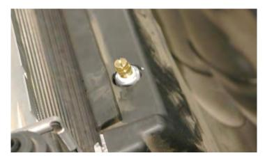
203. NOTE: If your vehicle had the soft rubber air deflector removed in step #194, this will already be done. If not, then now remove just the center bolt in the spoiler with a 10mm socket wrench as shown.
