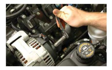
174. Connect the fuel line to the supercharger fuel rail manifold barb. Test the line by pulling firmly; you should not be able to remove the fuel line without using the fuel line removal tool.
