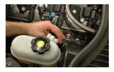
38. On the passenger side of the intake manifold behind the throttle body, remove the PCV hose by pressing the release clip and pulling free. Repeat on other end of the hose.
