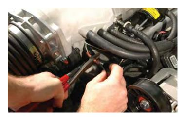
272. Use a heat gun or a hair dryer set on high to shrink the connectors onto the wire insulation. Shrink the plastic covering of the connector until the plastic covering has shrunk tightly around the wires. Crimping the connector alone is not enough to insure a permanent connection; you must shrink the plastic covering!
