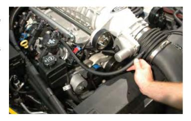
266. Connect the supplied throttle body cable extension to the OEM throttle body harness plug.
