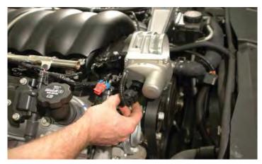
31. Disconnect the Manifold Absolute Pressure (MAP) sensor connector.
