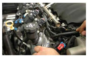
29. Disconnect the EVAP solenoid electrical connection.
