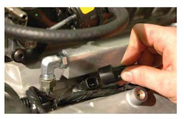
165. Mount the modified coil packs using the stock hardware, and torque the mounting bolts to 106 in-lbs. Verify your torque wrench settings.
