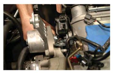
117. Install the pulley removed onto the new tensioner and torque the bolt to 40 ft-lbs. **Verify your torque wrench settings.**
