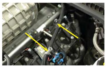
173. Route the split-loom covered cable between the coil packs and fuel rail. Attach the final mounting post to the stock location at the front of the driver side valve cover. Attach the eye terminal to the alternator using a 13mm wrench. Replace the cover on the terminal.
