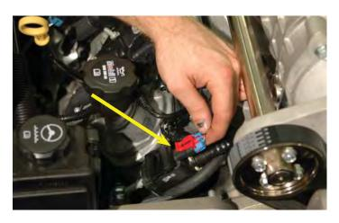
172. Remove these two alternator cable mounting clamps from the wire loom. The front clamp will remain in place and be utilized.
