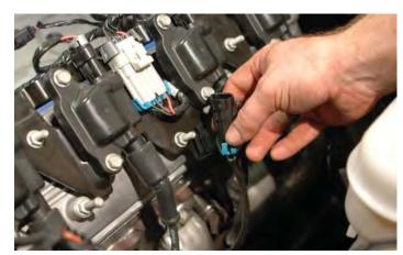
135. Disconnect the coil plug control connections from both sides of the engine.
