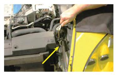
52. Remove the radiator cover and set it aside for a modification in a later step.
