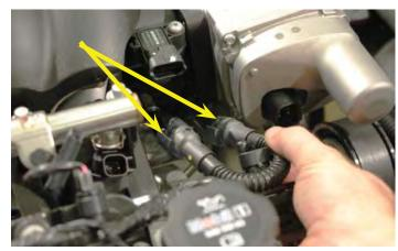
39. Release the fuel line safety clip. After removing the clip place some shop rags or towels under the fuel line in preparation for removal.
