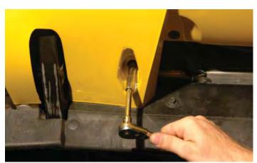
248. Bolt the brake cooling duct back to the original location in the wheel well using the stock hardware, and insert the push pin rivet back in the front to cowl splash shield location.
