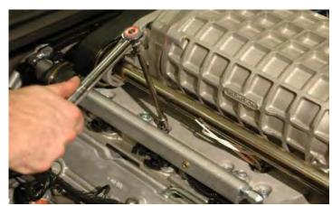
155. Use a 14mm wrench to remove the idler pulley directly below the supercharger inlet.
