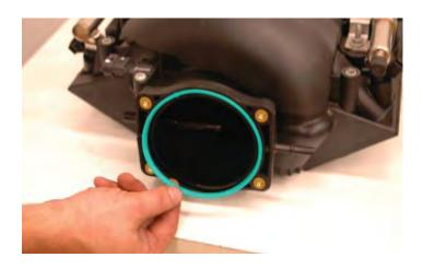
142. Install the throttle body gasket into the groove on the supercharger inlet manifold.
