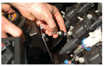
209. Add the supplied nut to mount the front of the reservoir bracket to the existing stud just behind the center of the coil bracket oxygen sensor plugs. Tighten using a 10mm wrench.
