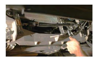
64. Swing the power steering cooler out and forward toward the driver side out of the way.
