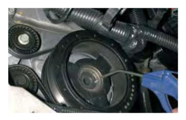
76. Place beads of Green Loctite on the two supplied hardened roll pins, and then insert them into the drilled holes. The use of a small hammer and punch may be necessary to tap the pins in. (Make sure that the pins are in far enough that they do not touch the balancer bolt.)
