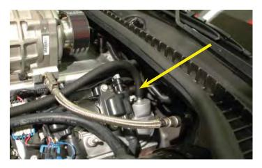
180. Route the hose forward below the fuel line, parallel to the brake booster hose. Connect to the barb adjacent to the brake booster hose you just installed.
