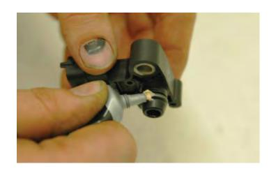
146. Install the sensor in its new location at the passenger side rear of the supercharger manifold and drop the split-loom spaced bolt into the mounting hole.
