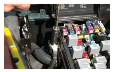
229. Replace the nut incorporating the large "eye" terminal of the red wire from the fuse holder of the intercooler wiring harness and secure using the 13mm wrench.
