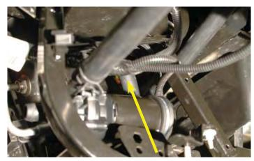
221. Connect one end of the provided straight 3/4" hose to the inlet barb on the intercooler pump using a supplied spring clamp. Route the other end up and into the engine compartment as shown.
