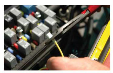
236. Plug the "spade" connector onto the fuse tap of the TCM-Trans fuse.
