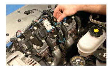
134. Unclip the receiving end of the oxygen sensor plug from the mounting slot on the coil bracket.
