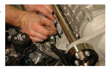
154. Torque the supercharger manifold bolts, working from the center out in a crisscross pattern to 106 In-Lbs. (10 Nm) using a 10mm socket and an inch pound torque wrench. Verify your torque wrench settings.
