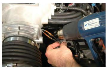
273. Cover the black and white wires using the provided split loom all the way back to the point where the white wires enter the supercharger lid. Zip tie your wires to ensure that they cannot be damaged by the supercharger serpentine belt, allow for lateral torque movement of the engine with the air box. Tape the junctions of your split loom.
