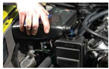
279. Fill the radiator reservoir with a 50:50 mixture of purified water and GM approved engine coolant only. After the initial start-up and the engine has come to operating temperature, recheck the fluid level in the reservoir and all the hose connections.
