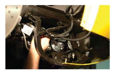
193. Remove the five 7mm bolts at the tail end of the nose cover and set aside for later re-installation.
