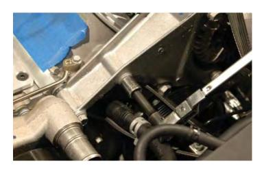
128. Remove the hose and clamp from the coolant vent "T" fitting.
