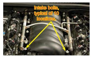
43. With the help of an assistant, feed the brake booster valve and hose as you carefully remove the intake manifold and set it aside.
