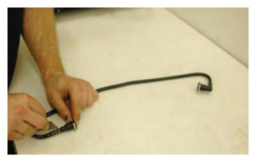
183. Connect the 90° elbow to one end of the supplied 5/16" hose. Use the supplied black spring clamp to secure the connection.
