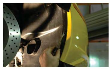
187. Remove the two 7mm bolts and one 10mm bolt that secure the passenger side end of the spoiler to the splash panel and frame with a socket wrench.
