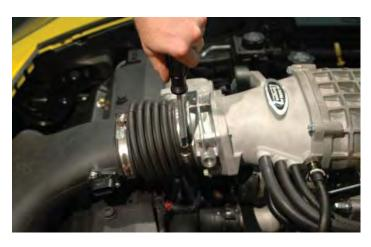
264. Press the push pin rivets of the air box assembly into the grommets you just installed. They should pop right in and lock the airbox in position. Removal just requires a firm tug on the airbox when you need to change the filter.
