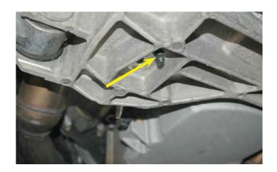
62. Using a suitable pry bar, pry down the sub-frame at the front two mounting points. Temporally push a metal or wooden wedge approximately 3/8" thick between the frame and sub frame at these points.
