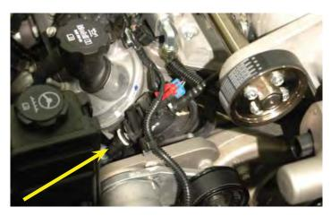
185. Connect the other fitting removed from the OEM hose to the free end using the supplied black spring clamp and connect to the remaining EVAP barb on the driver side of the supercharger inlet as shown.
