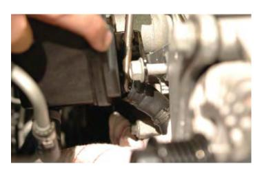
104. Remove the small hose from the bottom of the reservoir. Be careful of dripping fluid, use a shop towel and dispose of properly.
