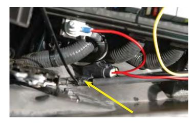
231. Remove the nut from the ground post by the passenger side hood shock mount near the radiator using a 10mm wrench.
