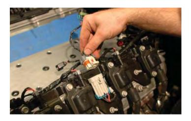
136. Disconnect the spark plug wires from the coils.
