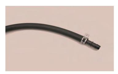
120. Install the 5/8" hose with the connector into the end of the large power steering hose to the pump. Secure the connector with the original spring clamp.
