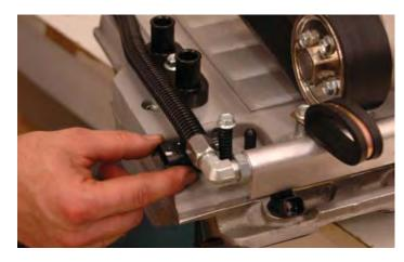
147. Install the two intake manifold gaskets supplied onto the recesses in the manifold face.
