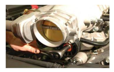
156. Temporarily pull the front fuel crossover line (encased in split loom) out in front of the pulley mounting flange as shown.
