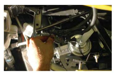
192. Use a 10mm wrench to remove the horn assembly from the diagonal fascia sub-frame mounting location.
