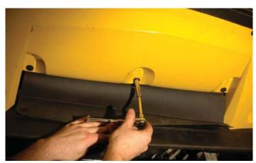
195. Remove this push rivet from the inside of the nose cover sub frame. This rivet is adjacent to the bolt removed at the recess on the passenger side of the nose cover.
