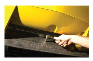
204. NOTE: If your vehicle had the soft rubber air deflector removed in step #194, this will be done at a later moment. If not, install the Heat Exchanger retaining bracket with the bolt removed in the previous step. Ensure that the foam pad is contacting the lower tank of the heat exchanger and tighten the bolt securely.
