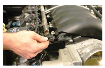
32. Use a shop knife to cut the tape that secures the wiring harness to the fuel rails in four locations.
