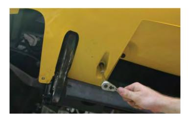
194. NOTE: If your vehicle has the soft rubber air deflector between the nose fascia (as shown in this picture) and the front frame cross member; there will be three 10mm bolts attaching the rear edge of the air deflector to the frame cross member that need to be removed as well. Temporarily remove the soft rubber air deflector from the vehicle and set aside for later reinstallation.
