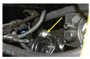
243. Reconnect the horn plug to the horn assembly.
