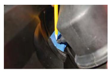
260. Remove the bellows and airbox, use an awl or center punch to mark through the tape onto the splash shield/air deflector.
