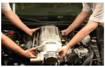
153. Remove the black plastic sleeves that hold some of the intake bolts up and start all ten intake bolts by hand. Do not tighten until all the bolts are started. (Be careful not to cross thread the bolts.)
