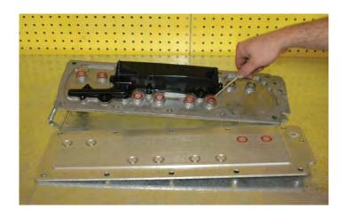
96. Install the new valley cover. Fasten with the supplied flathead bolts using a 5mm Allen socket and wrench. Torque the bolts to 18 ft-lbs. Verify your torque wrench settings.
