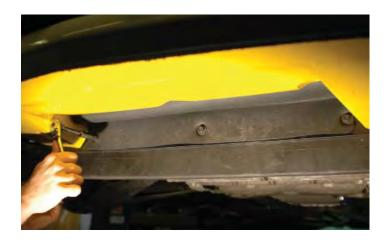
254. Place a strip of light colored tape on the driver side of the upper grooves in the splash shield/air deflector in front of the radiator/heat exchanger as shown.
