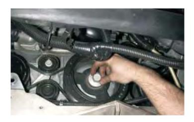
78. Using a 24mm socket tighten the new harmonic balancer bolt according to General Motors specifications. Tighten to 50 Nm (37 ft-lbs) then tighten an additional 140° using a torque angle meter.
