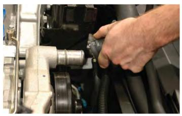
101. Using a power steering oil suction tool, turkey baste bulb, hand soap pump, or whatever you can improvise with to remove the fluid from the power steering reservoir and put into a disposable container. (Old fluid can be disposed of at an oil recycling center.)
