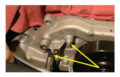
110. Use a die grinder, reciprocating saw, hacksaw, or what have you to cut off the two bosses shown level with the face of the surface of the boss from the removed bolts.
