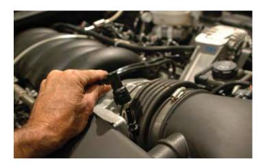
22. Use an 8mm nut driver or flathead screwdriver to loosen the clamp on the bellows to the throttle body.
