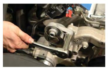
88. Remove the coolant hose from the vent pipe.
