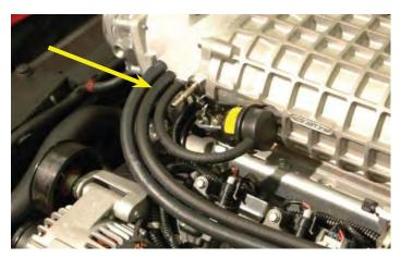
181. If your vehicle is equipped with a Vacuum Controlled Exhaust Baffle, attach one end of a cut-to-fit 3/8" hose on the firewall barb. Cut the existing bypass hose as shown, insert the provided "T" in the cut ends and connect the other end of the 3/8" hose to the remaining "T" connection as shown. No clamps are necessary.
