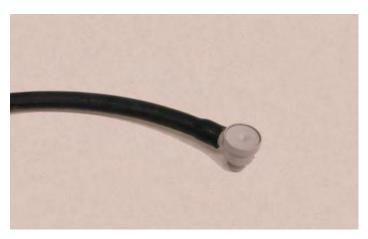
177. Plug the brake booster valve into the stock location on the brake booster canister.
