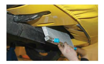
202. Move the heat exchanger around until the air-bleed valve appears in the newly created hole in the radiator shroud.
