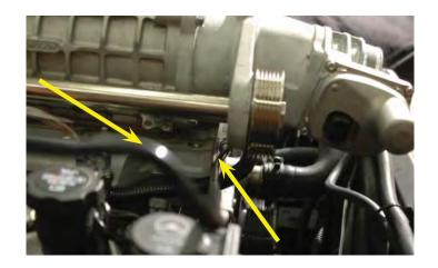
158. Plug the EVAP sensor connection onto the EVAP solenoid upper barb.
