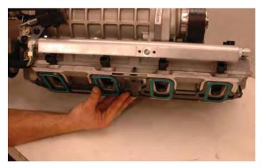
148. Install the fuel manifold O-ring into the recess on the fuel rail, use some of the Lubriplate lubricant supplied.
