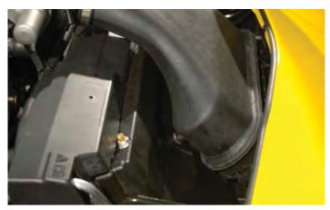
265. Cut a section of the provided 3/8" hose to 18" in length. Connect one end of the hose to the PCV hose barb at the front passenger side of the valve cover by the oil filler spout. Connect the other end to the barb on the supercharger inlet as shown.
