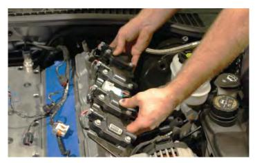
139. Use a small flathead screwdriver to unsnap the plastic wire covers and remove the covers from the coil brackets.
