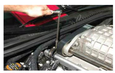
216. Place the clamp around the two hoses from the supercharger intercooler and tighten in place. The spacer remains between the clamp and the supercharger lid. Tighten the bolt to 106 in-lbs; be sure to verify your torque wrench settings.
