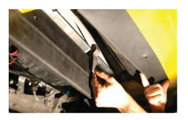
253. Use the remaining three 10mm bolts to attach the frame end of the soft rubber air deflector incorporating the heat exchanger mounting bracket in the center hole. Ensure that the foam pad of the bracket is contacting the lower tank of the heat exchanger and tighten the bolt securely.
