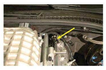
160. Relocate the fuel crossover line back behind the idler pulley mounting flange from where you removed it in step #156.
