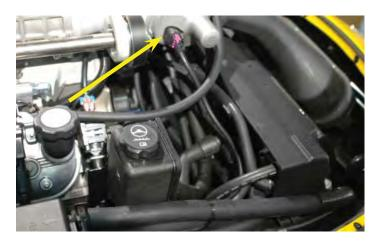
268. Zip-tie the wire extension to the existing hoses to keep the wiring free from the belt line.
