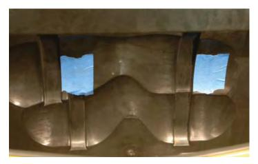
255. Assemble the new airbox using the stock "bellows" on the throttle body end, and the provided screws and spacers with the stock air filter on the intake end. The spacers go between the stock air filter and the air box. Remove the MAF sensor from the OEM airbox and attach to the new airbox location. This is the completed air box assembly. Note the spacers between the airbox and the OEM air filter.
