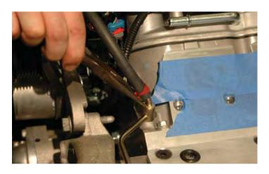
132. Connect the oil pressure sensor plug to the oil pressure sensor on the new valley cover.
