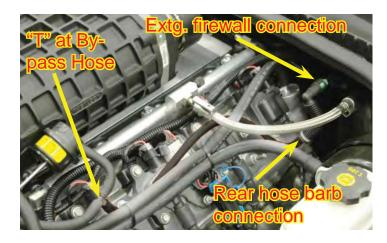
182. Remove the two fittings from the disconnected EVAP hose removed earlier using a sharp blade to split the plastic. Be careful to not cut the fittings.
