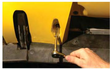
251. Use the three stock 7mm bolts to secure the remaining (center) nose fascia locations, incorporating the soft rubber air deflector removed in step #194 as shown.
