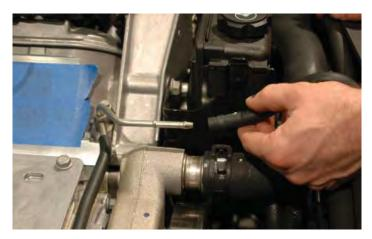
89. Remove the vent pipe with a 10mm socket wrench. Ensure that the O-ring gaskets under the vent pipe blocks do not stick to the cylinder heads. If so, remove them as new gaskets are supplied.
