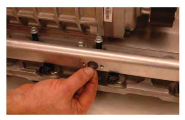
149. Next install the fuel manifold to the fuel rail using the supplied bolts. Tighten and torque the bolts with a 10mm socket and torque to 106 in lbs. Verify your torque wrench settings.
