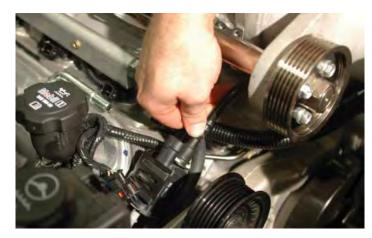
159. Plug the other end of the EVAP tube onto the barb at the rear of the driver side valve cover.
