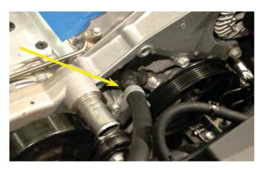
121. Pass the 5/8" hose through the center of the new serpentine drive belt.
