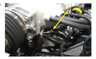
270. Connect the MAF plug extension to the MAF plug you installed earlier in the new air tube.
