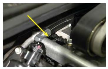
171. Connect the EVAP sensor plug to the EVAP solenoid.
