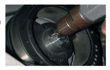
72. Using compressed air, blow the drill shavings out of the holes.
