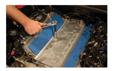
94. Remove the stock valley cover. The gasket will be reused, the original valley cover will not. Inspect the gasket for any damage and then re-install just the gasket, note that it will only fit correctly in one position.
