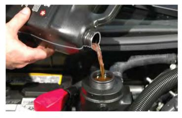
281. Using a straight blade screwdriver. Open the bleed valve to let any trapped air escape form the intercooler system. Some coolant will be lost when bleeding the system. Add coolant as necessary to the reservoir and continue to bleed the system until you can get a steady stream of coolant from the valve for over one minute. Check the intercooler reservoir level and re-open the bleed valve as needed.
