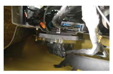
276. Reverse the steps, and re-install the plastic panel covering the ECM and TCM. This was removed in steps 5-7.
