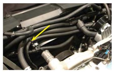
125. Connect the end of the 3/8" hose to the small barb on the power steering reservoir using the supplied green clamp (the reservoir is shown lifted for clarity).
