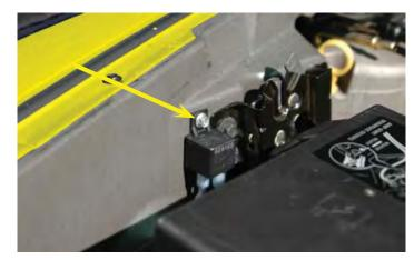
239. Route the plug end of the intercooler pump harness forward and down to the intercooler pump and connect to the terminal near the clamp on the forward end of the pump as shown.
