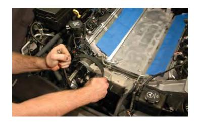
86. Use a 15mm wrench to remove the pulley from the tensioner assembly. Set this pulley aside for later installation with the new tensioner.
