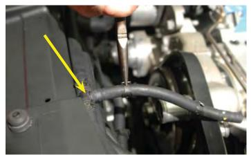
129. Connect the new 1/4" coolant hose to the coolant vent "T" fitting with a provided red clamp. Route the hose along the same path as the PS hoses to the barb on the coolant vent pipe.
