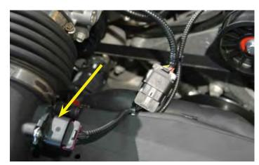
271. There are two black wires pulled off from the extension. Strip ½" off the ends of these two wires and the two white wires from the IAT sensor exiting the supercharger lid. Using the supplied crimp connectors, crimp the black wires to the white wires. It doesn't matter which wire goes to which.
