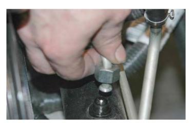
80. Remount the power steering cooler assembly to the original location and fasten using the original hardware. Torque the bolts to 106 in. lbs. Verify your torque wrench settings.
