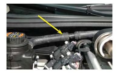
214. Cut 2" off the short end of one of the supplied 3/4" x 4" x 36" elbow hoses. Install this short end onto the driver side barb of the supercharger intercooler using one of the supplied worm gear clamps. Route this hose over to the passenger side and forward between the reservoir and the coil brackets.
