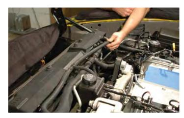
51. Using a 10mm socket wrench, remove the two bolts on each side of the radiator cover.
