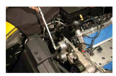
116. Place the other angle from the tensioner brace bracket package on the back of the long bolt you just tightened. The Long slot should align with the long slot on the angle mounted earlier on the power steering reservoir bracket. Tighten in place aligning the two angles together. Use the provided nut and bolt to tie the two angles together, anchoring the tensioner assembly.
