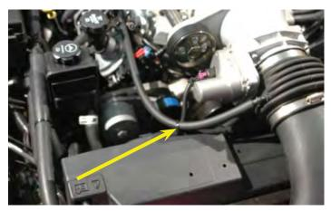
269. Route the two white IAT wires on the driver side of the supercharger lid forward just above the fuel crossover line to the driver side of the engine.
