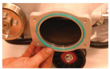
143. Install the throttle body onto the inlet manifold using the original bolts. Tighten the bolts with a 10mm socket and torque to 106 In-Lbs (12Nm). Verify your torque wrench settings.
