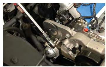
115. Install the tensioner with the provided long 19mm bolt in the tensioner package. Torque the bolt to 50 ft-lbs. Again, verify your torque wrench settings.
