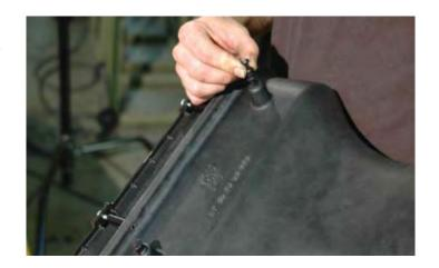
258. Push the bellows end of the air box onto the throttle body and loosely tighten the clamp.
