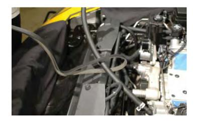
122. Route the 5/8" power steering hose forward along the fan shroud, following the same path as the coolant lines toward the passenger side of the vehicle, cut to fit and connect to the large barb on the power steering reservoir using the provided clamp.
