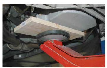
68. When raising the engine with the floor jack, take care to watch the clearance between the back of the engine and the fire wall, so as not to damage any of the components on the fire wall.
