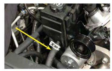
123. Connect the length of 3/8" hose to the barb on the bottom of the power steering cooler. Secure the hose with the green clamp supplied.
