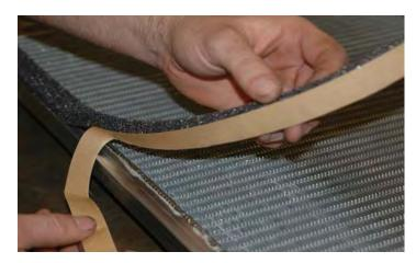
199. Apply a small piece of the foam strip to the Heat Exchanger Retaining Bracket.
