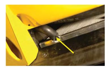
220. After passing through the hole in the splash panel, route the hose up and into the engine compartment prior to reaching the intercooler pump.
