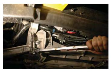
85. Remove the accessory serpentine belt by rotating the tensioner bolt with a 15mm wrench. Once the belt has become slack, pull the belt off an idler pulley and then remove the belt, this will not be reused.
