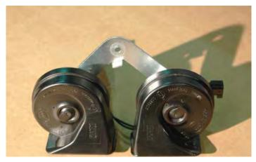
241. Remove both horns from the bracket using a 10mm wrench. And remount to the bracket as shown in this picture. The horns will now be facing forward instead of down and on the opposite side of the bracket. The horn plug will now be toward the rear and facing up.
