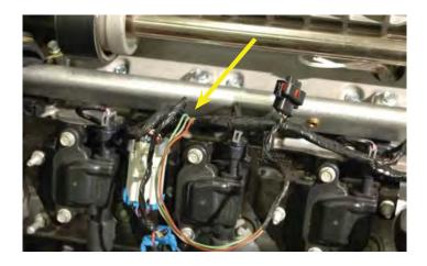
170. Route and tuck the MAP sensor wires back along the fuel rail and plug into the map sensor at the rear, passenger side of the supercharger lid.
