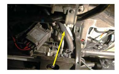
222. Cut the remaining end of the hose from the intercooler pump inlet barb to fit to the discharge barb on the intercooler reservoir. Clamp onto the barb using one of the supplied worm gear clamps.
