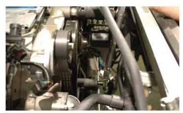
71. Using a small or angled 3/8" drill and the supplied drill bit, insert the drill into the guide holes and drill to the second step of the drill bit. (Make sure that you drill all the way to the second step.)
