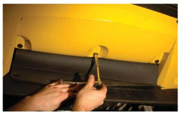
252. This shows the center spoiler mounting hole which will be the location of the heat exchanger mounting bracket. We will incorporate this bracket with the re-attaching of the back edge of the soft rubber air deflector.
