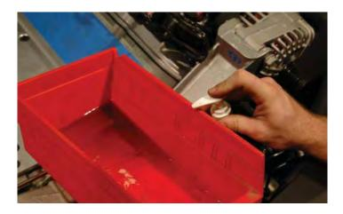
102. Using a 15mm wrench, remove the two bolts that secure the power steering fluid reservoir to the alternator bracket.
