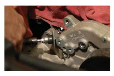
112. File the bottom of the upper radiator hose barb casting by the water pump pulley for additional belt clearance. This will be about 1/10" (100/1000) at the outside edge and parallel back toward the face of the casting.
