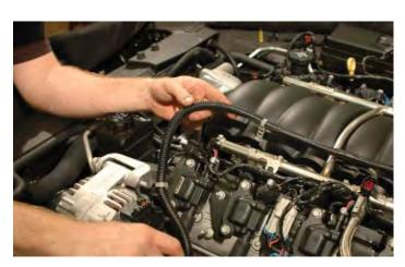
36. Free the battery cable from the intake manifold and lay it aside.
