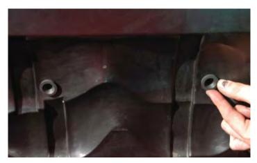
263. Attach the air bellows of the air box assembly back onto the throttle body and tighten using a flathead screwdriver or 8mm nut driver. Tighten firmly in position.
