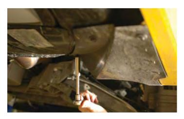
8. Removing the inner fender panel will expose the vehicles operating computer. This is high in the fender well. Remove the two 10mm bolts that anchor the computer to the fender mounting bracket. Pull the computer off the locating pins. The computer is now free to drop down.
