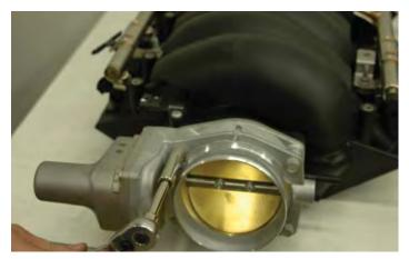
141. Carefully remove the throttle body gasket from the intake manifold.
