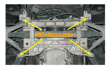
60. Loosen the four front sub-frame nuts until the bottom of the nut is even with the end of the threads on the bolt. The gap between the washer and the sub-frame should be approximately ½".
