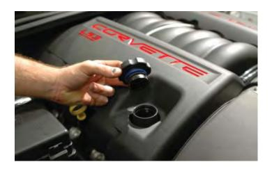
18. Remove the engine/coil covers by pulling up firmly on them. The covers will not be reused.
