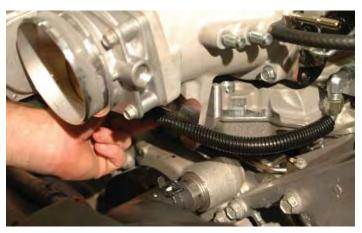
157. Route the stock EVAP tube under the supercharger inlet where the fuel crossover was located as shown, and then route the long straight shaft back on the driver side of the engine between the fuel injectors and valve cover.
