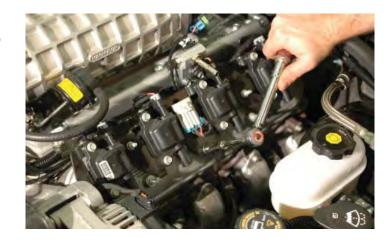
166. Connect the oxygen sensor coil pack plugs in their original location. Engage the mounting clip in place at the bottom center of the coil pack.
