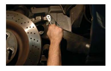
249. Install the fender well splash shield using all the stock fasteners (this is a reversal of steps 207-208).
