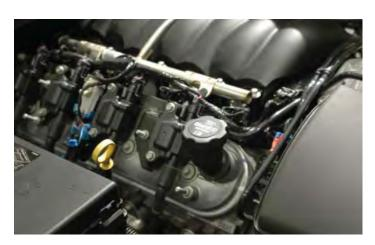
20. Remove the Mass Air Flow meter (MAF) connector from the airbox by pulling up on the grey release trigger and squeezing the connector.
