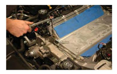
92. Use a 1-1/16" wrench to remove the oil pressure sensor from the engine valley cover.
