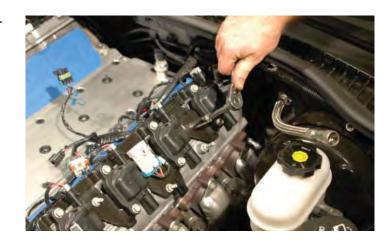
138. Remove the coil brackets for modification.
