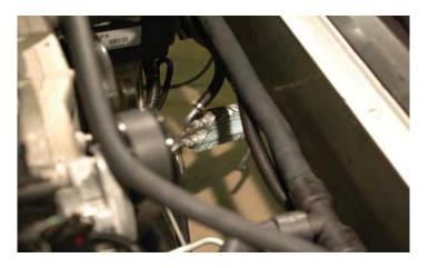
65. Using a 16mm wrench, remove the power steering line attached to the top of the steering rack. Use a shop towel to catch any fluid lost.
