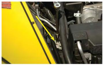
232. Route the black ground wire from the intercooler pump harness to the stud you just exposed and add the "eye" terminal to the ground, replace the nut and tighten with a 10mm wrench.
