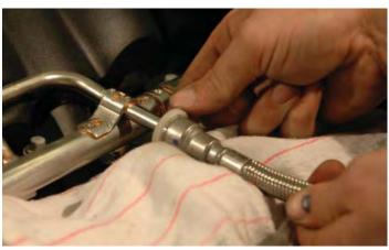
41. If you have, or can improvise, we recommend that you plug both the fuel line and the fuel line barb on the fuel rail to contain fuel seepage. Use shop towels to catch any dripping fuel and dispose of properly.
