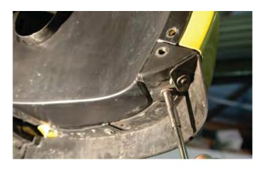
188. Remove the front driver side splash panel assembly from the vehicle. You will need to separate the pieces for re-assembly later.
