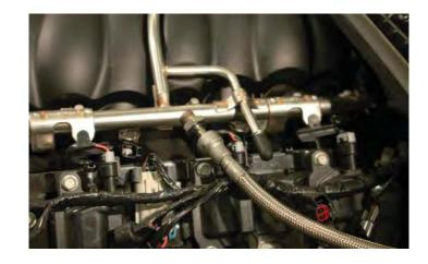
42. With an 8mm socket wrench remove the ten intake manifold bolts.
