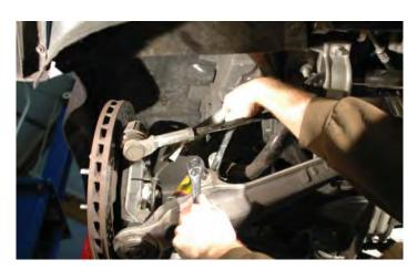
48. From under the vehicle, remove the four bolts that secure the sway bar brackets to the chassis with a 13mm socket wrench
