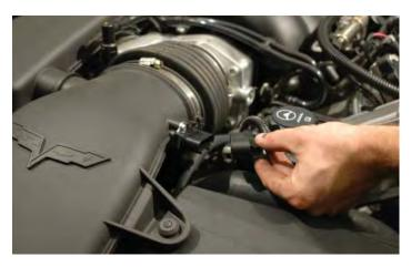
21. Remove the PCV inlet tube from the air filter bellows by pushing up on the release lever. The tube will not be reused.
