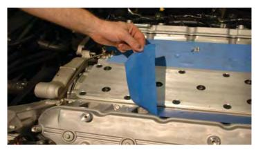
151. Spray silicone or some mild soap and water solution on the cylinder head surface to lubricate. This makes the intake manifold slide around a little to help line up the holes. (Do not use anything that will damage the intake gaskets, petroleum based products, etc.)
