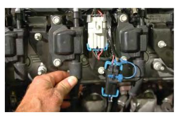
168. Before you tuck the wires of the injectors harness below the coil packs, remove the tape off the passenger side harness to about the center bolt of the coil pack. This is to free the MAP sensor plug from the harness where it will change direction and go to the rear of the supercharger.
