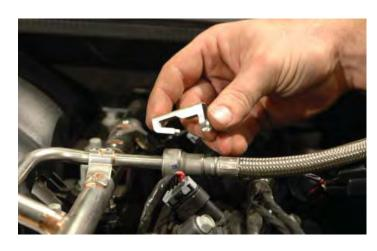
40. Use the fuel line removal tool to remove the fuel line from the fuel rail. To do this, first push the fuel line onto the barb firmly, hold in place while you insert the supplied fuel line removal tool into the fuel line. Push the tool into the fuel line releasing the spring clip and pull the fuel line off of the fuel line hose barb.
