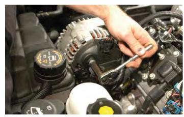
35. Pull up on the anchors that secure the battery cable to the intake manifold and fuel rail (three locations).
