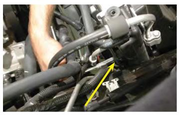
57. Remove the bolt near the bottom on the driver side with a 10mm socket wrench. The fan shroud should now be free to remove.
