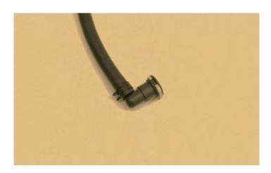
184. Connect the 90° elbow to the bottom barb of the EVAP sensor, and route the free end of the hose under the EVAP sensor, below the supercharger inlet to the driver side of the engine.
