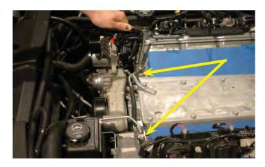
90. Install the new O-ring gaskets on the vent pipe blocks using some of the supplied Lubriplate lubricant to hold them in place.
