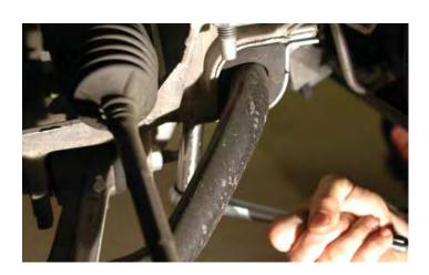
84. 84. Torque the sub-frame, the sway-bar connections and motor mounts to the torque values below. Torque Specifications:
