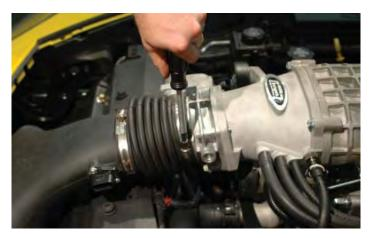
259. Use a sharp pencil or pen to mark around the strike of the push pin rivet mounting posts onto the light tape (you placed on the splash shield/air deflector earlier). Be careful to not move the air box between marking each side of the air box push-pin mounting posts or installation will be difficult.
