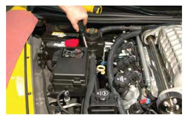
223. Route the two ¾" x 2" x 36" elbow hoses (one from the driver side of the supercharger intercooler and one from the heat exchanger passenger side barb) to meet at or near the power steering reservoir. Cut the hoses to fit and join using one of the supplied hose couplings (mender) and supplied spring clamps.
