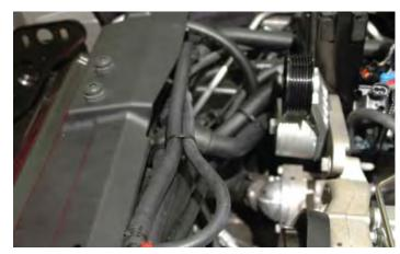
131. Connect the hose from "T" fitting to the barb on the coolant vent pipe. Secure the hose with a red clamp provided.
