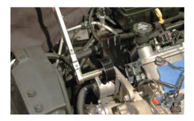
118. Slide the power steering reservoir into place on the new mounting bracket.
