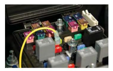
237. Note where the wire lays over the fuse center edges and cut notches in both the base and the cover so as to not have the wire get pinched with the lid opening and closing which could compromise the insulation.
