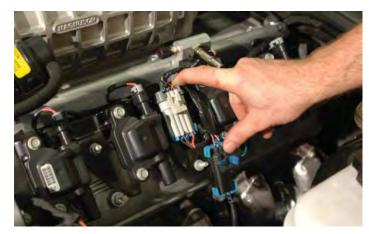
167. Connect the plug wires to the coils.
