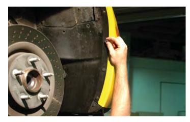
247. Re-attach the nose fascia at the bottom using all the stock fasteners, tighten securely.
