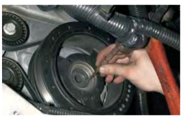
77. Install the new supplied factory GM harmonic balancer bolt.
