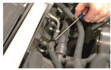
55. Locate the cooling fans electrical connector under the wiring harness located on the fan shroud. Squeeze the connector firmly and pull the connector free as shown.
