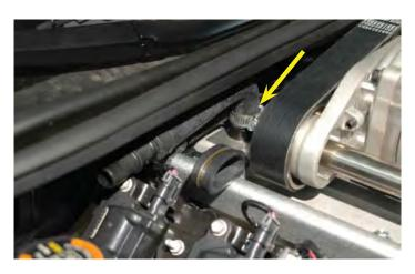
213. Cut 2" off of the short end of the other supplied ¾" x 4" x 18" elbow hose. Cut the long end off to fit where it will join the hose you just installed on the supercharger intercooler. Use the supplied spring clamps on the coupling end and worm gear clamps on the reservoir end and supercharger inlet end. Tighten firmly.
