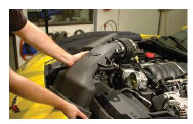
24. Disconnect the EVAP intake tube on intake manifold by pushing in on the white release trigger and pulling the connector free.
