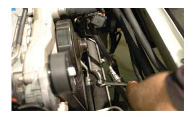
66. Unplug the oil pressure sensor electrical connection at the rear of the valley cover.
