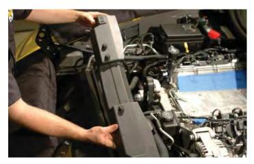
53. Un-clip the coolant hoses from the three clips on the fan shroud.
