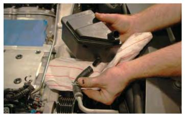
105. Cut or open the factory pinch clamp from the top barb on the power steering cooler. Pull the hose off the barb quickly placing your thumb or finger over the end of the hose to minimize the mess. Use shop towels to catch any residual fluid. This entire section of hose and hardline will not be reused.
