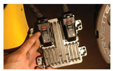
275. Re-install the computer on the mounting bracket using the original fastener and a 10mm socket wrench. Note: If your vehicle has an automatic transmission, you will also need to re-install the transmission control computer located on the back side of the mounting bracket.
