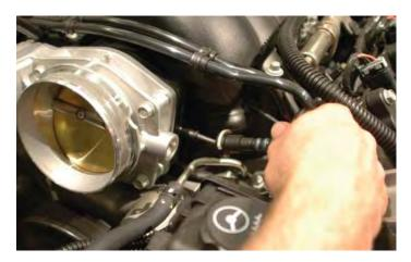
25. Release the other end of the tube at the bottom of the EVAP solenoid by pushing in on the release trigger.
