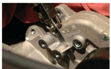
111. Test fit the new tensioner bracket and assembly to check for full travel. You will need to adjust the cut at the passenger side boss as necessary. Roughly, you will be grinding from the bolt hole at an angle back toward the water pump casting on the side nearest the passenger side fender. Test your cut using the new tensioner assembly and adjust as necessary.
