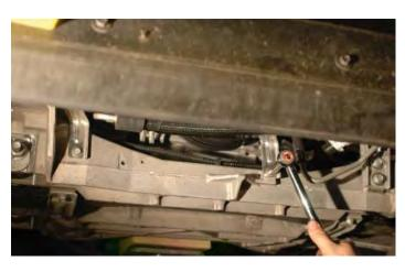
81. Reinstall the fan assembly. Use care to not damage the radiator core, and clip the fan assembly back into place. Install the two bolts that held it into place and reconnect the fan electrical connection. Clip the wiring harness and coolant lines back into their original locations on the fan shroud. (This is a reverse of steps 50-58)
