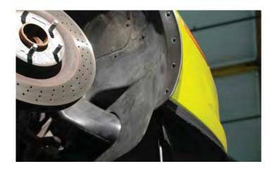
250. NOTE: For vehicles with the soft rubber air deflector follow the next four steps. If your nose fascia was attached in step #247, skip to step #254. Re-attach the underside ends of the nose fascia as shown using the two outside 7mm bolts, tighten securely.
