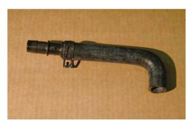
212. Install the short end of the hose you just modified to the passenger side barb of the supercharger intercooler. The hose coupling (mender) should be facing the passenger side of the vehicle.
