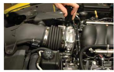
23. Pull up firmly on the air box assembly to separate from the three mounting grommet pins and remove from the vehicle.
