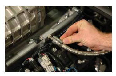
176. Remove the OEM brake booster valve on the stock hose from the OEM intake manifold removed earlier. Install the brake booster valve just removed on one end of the supplied 11/32" hose. Use some lubrication to help with the tight fit.
