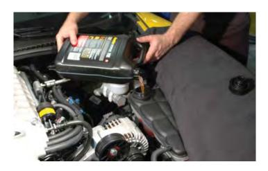
280. Fill the intercooler reservoir with a 50:50 mixture of purified water and GM approved engine coolant only. The intercooler system will hold approximately 6 quarts of liquid. Fill the reservoir until the fluid level comes to about one and a quarter inch from the top edge of the filler neck.
