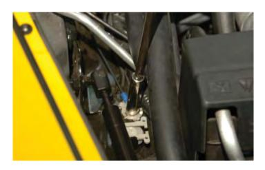
233. Use the legend on the inside of the fuse center lid to locate and remove the 10amp TCM-Trans fuse. Install the provided fuse-tap onto one leg as shown.
