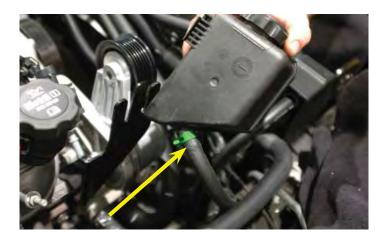
126. Using a pair of pliers to squeeze the stock spring clamp, rotate the coolant line shown where it meets the water pump housing. Rotate the hose so that it will not contact the tensioner mounting bolt and release the clamp to hold it the new position. Alternately you can loosely zip tie the hose together with the large power steering hose you just ran.
