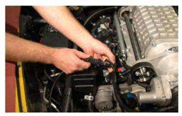
267. Route the other end of the harness extension under the power steering reservoir along the radiator and connect to the throttle body.
