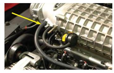
179. Cut a section of the supplied 3/8" hose to 26-1/2" in length. Connect one end of the hose to the driver side PCV barb at the back of the driver side valve cover. This barb is covered with a rubber cap that must be removed first.
