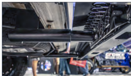
Designed to absorb rear impacts up to 5mph and avoid possible frame damage
