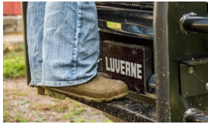
Built-in 4" diamond tread step for easy access under the hood
