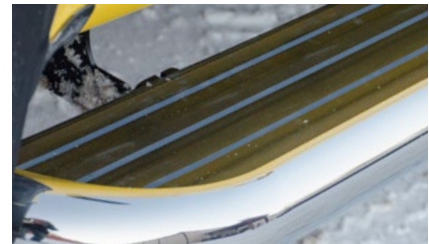
5" non-skid rubber treads for a safe, comfortable step
