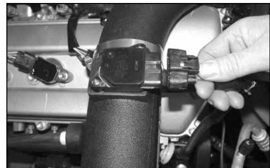
33. Reconnect the mass air sensor electrical connection.
