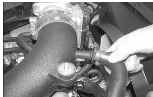
29. Install the original crank case vent hose onto the valve cover, then connect the opposite end of the crank case vent hose onto the K&N® intake tube.
