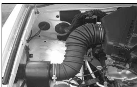
3. Loosen the hose clamps securing the intake tube to the air box and resonator.
