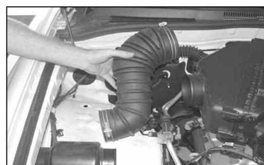
5. Remove intake tube from the vehicle as shown.
