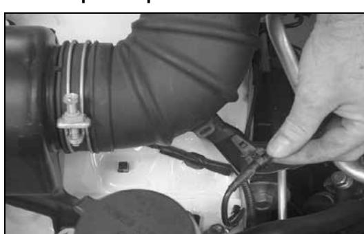
4. Pull the wire harness clip up to release from the intake tube.
