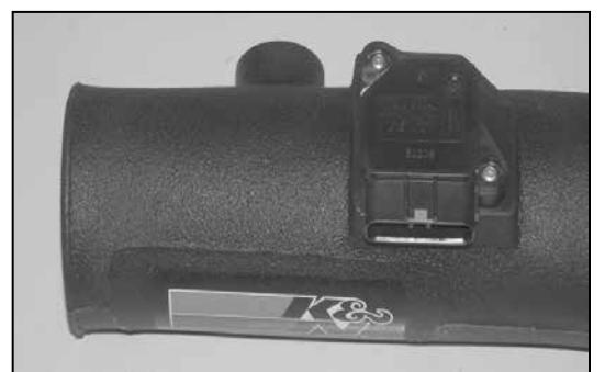
23. Secure the mass air sensor to the K&N® intake tube using the provided screws and spacers as shown.
