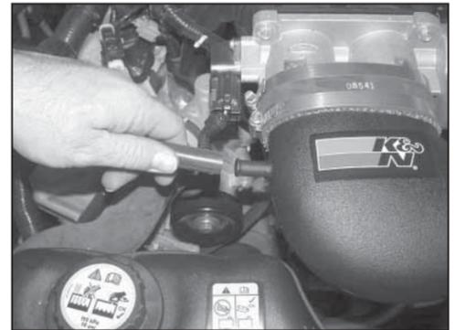
20. Install the supplied vent hose onto the vent port on the valve cover and then onto the K&N® intake tube as shown.
