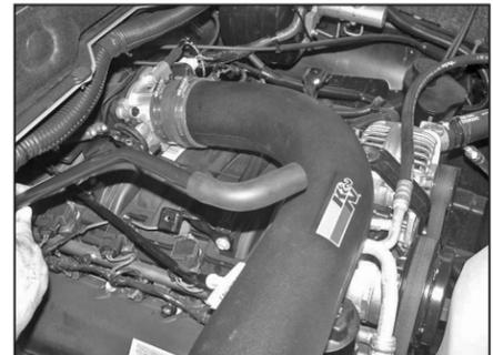
30b. On models that the crank case vent hose is connected to the passenger side valve cover, remove the factory 90° coupling hose from the plastic vent tube.
