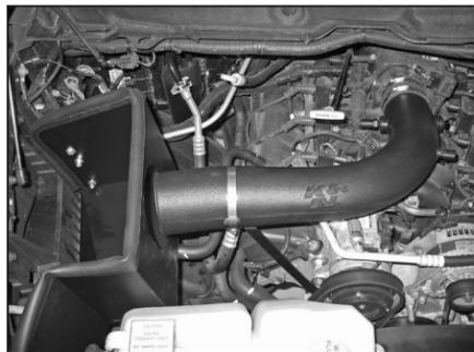
28. Install the K&N® intake tube into the silicone hose at the throttle body and align to the mounting bracket, secure the intake tube with the hose clamps provided.
