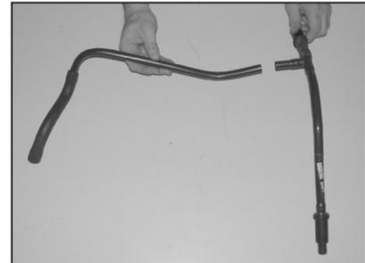
30c. Cut the crank case vent tube 1" from the "T" fitting as shown.
