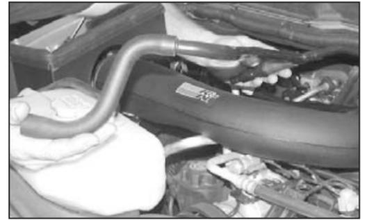
30a. On models that the crank case vent hose is connected to the "T" on the passenger side of the engine, remove the complete vent tube assembly from the rubber fittings in each valve cover as shown.
