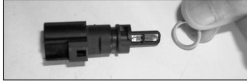
26. Remove the O-ring from the air temp. sensor as shown.
