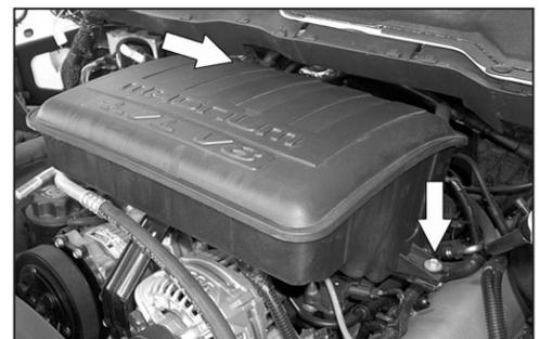
5. Remove the two 10mm bolts that retain the resonator box onto the engine.
