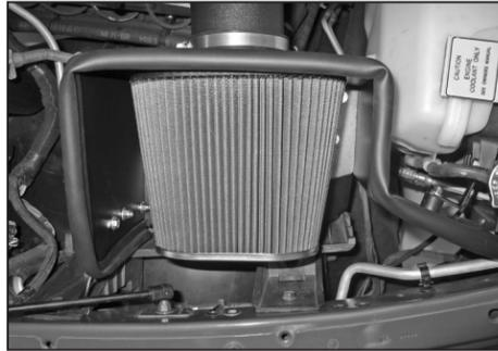
34. Install the K&N® [air filter](#) onto the intake tube as shown.
