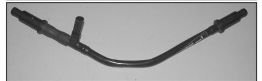
30d. Rotate the long side of the vent tube assembly 180° as shown.
