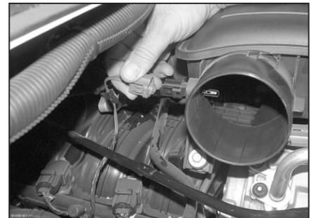
4. On models that come equipped with air temp sensors, unplug the air temp. sensor electrical connection as shown.
