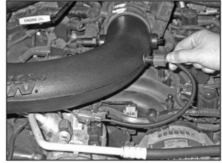
29. On models equipped with an air temperature sensor, connect the harness extension into the factory connector and then connect the open end onto the air temperature sensor.
