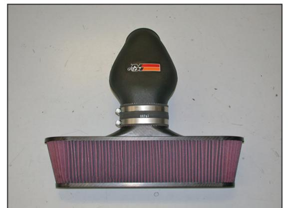
8. Install the K&N® intake tube onto the air filter as shown and secure with the provided hose clamp.
