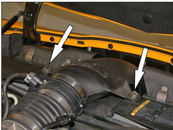
3. Loosen the hose clamp which secures the stock intake tube to the mass air sensor, then pull up to release the center locking pins in the intake tube mounting fasteners shown.
