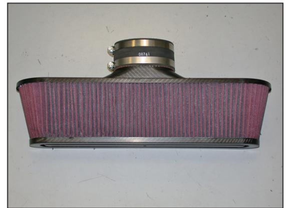
7. Install the silicone hose (08625) onto the air filter as shown and secure with the provided hose clamps.
