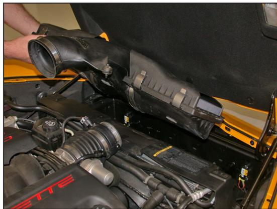
4. Pull up on the complete intake system to disconnect it from the air box mounting pins and then remove it from the vehicle as shown.
