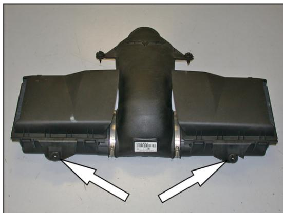
5. Remove the two rubber mounting grommets shown air box as shown.
