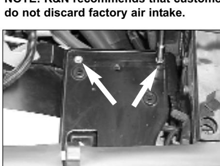
5. Loosen and remove the two air cleaner mounting tray bolts as shown.
