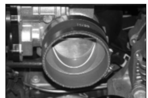
10. Install the silicone hose (08625) and hose clamps onto the throttle body as shown.
