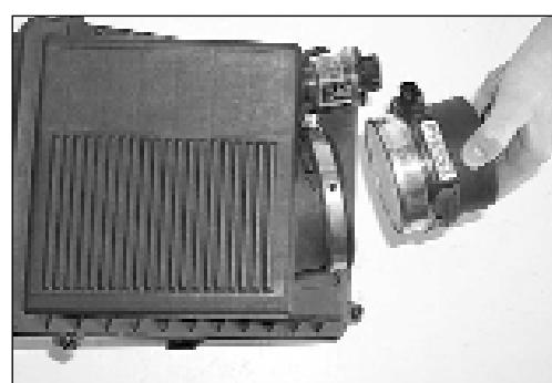
6. Loosen the hose clamp and remove the mass air sensor from the air cleaner.
