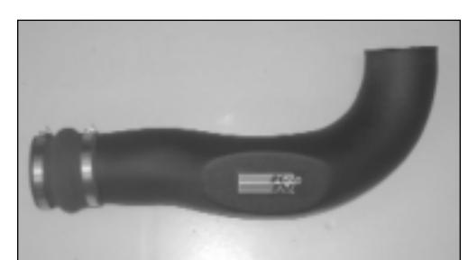
11. Install the silicone hump hose (08176) and hose clamps onto the K&N intake tube as shown.
