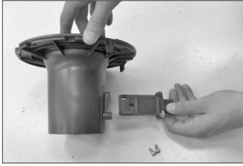
14. Remove the mass air sensor retaining screws and then remove the mass air sensors from it's housing as shown.
