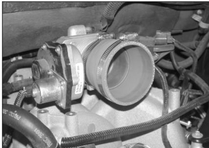
19. Install silicone hose (08724) onto the throttle body with the provided hose clamp as shown.
