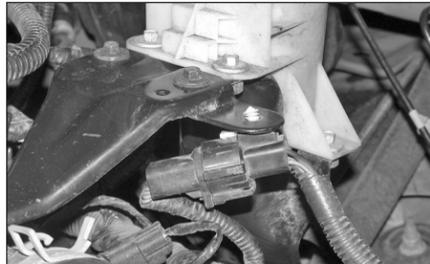
4. Unhook the secondary mass air sensor electrical connection from the power steering reservoir bracket, then unlock the electrical connection locking tabs and separate the electrical connection
