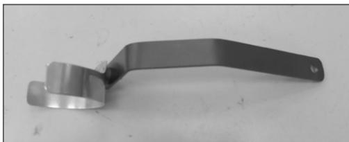
20. Install the saddle clamp onto the tube mounting bracket as shown using the provided hardware.
