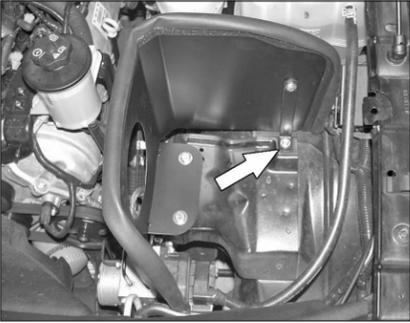
10. Install the heatshield as shown and secure with the provided hardware.
