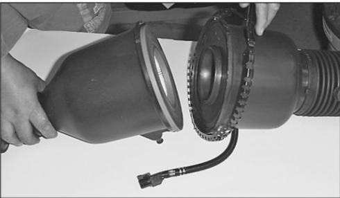
11. Open the air cleaner assembly and isolate the mass air sensor assembly.
