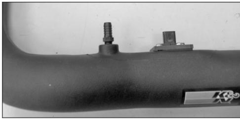
18. Install the provided 1/4" npt fitting into the K&N® intake tube as shown.
