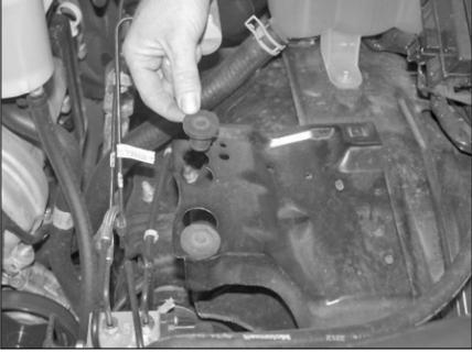
9. Install the provided nut inserts into the air box mounting holes as shown.
