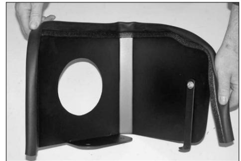
7. Install the edge trim onto the heatshield as shown.
