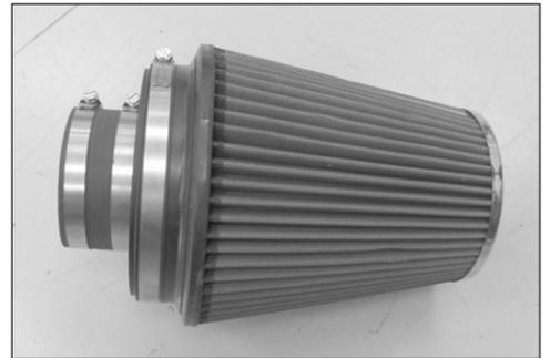
25. Install the silicone hose (08630) onto the filter assembly and secure with the provided hose clamp.
