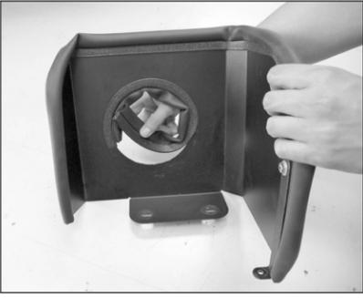
8. Install the edge trim into the hole in the heat shield as shown.
