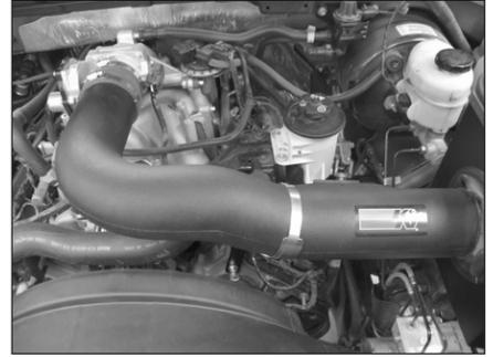
22. Install the K&N® intake tube into the silicone hose at the throttle body and onto the tube mounting bracket assembly. Secure with the provided hose clamps.
