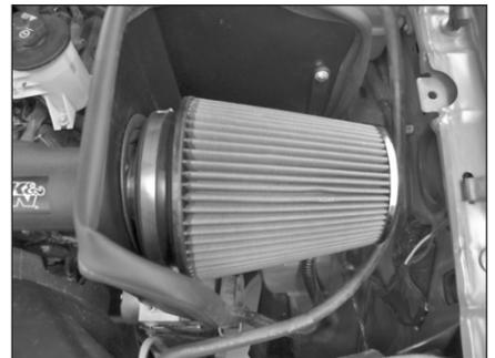
26. Install the filter assembly onto the K&N® intake tube and secure with the provided hose clamp.
