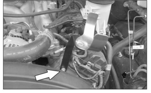
21. Install the tube mounting bracket assembly onto the 8mm stud protruding from the engine with the nut and washer provided.
