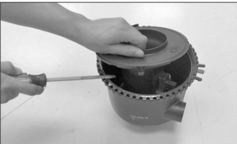
13. Using a flat blade screwdriver, push in and release the four clips that retain the mass air sensor retaining plate.
