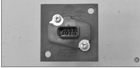
16. Install the mass air sensor into the adapter using the factory screws.
