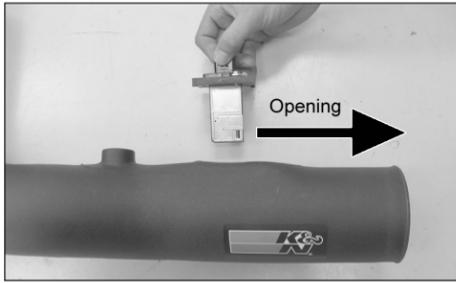
17. Install the mass air sensor assembly into the K&N® intake tube and secure with the provided hardware.
