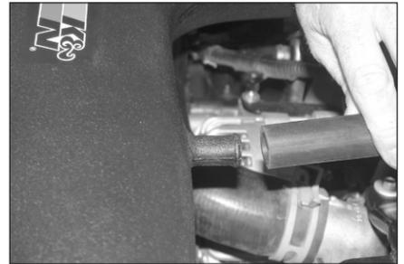
23. Install the provided silicone vent hose onto the valve cover and onto the K&N® intake tube as shown.
