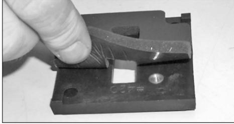
15. Remove the backing paper and install the mass air sensor adapter gasket as shown.
