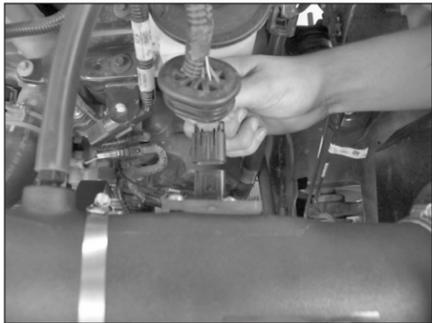
27. Reconnect the secondary mass air sensor electrical connection and then reconnect the mass air sensor primary electrical connection.
