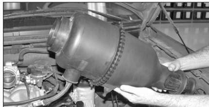
5. Pull firmly up on the air filter assembly to remove it from the mounting grommets.
