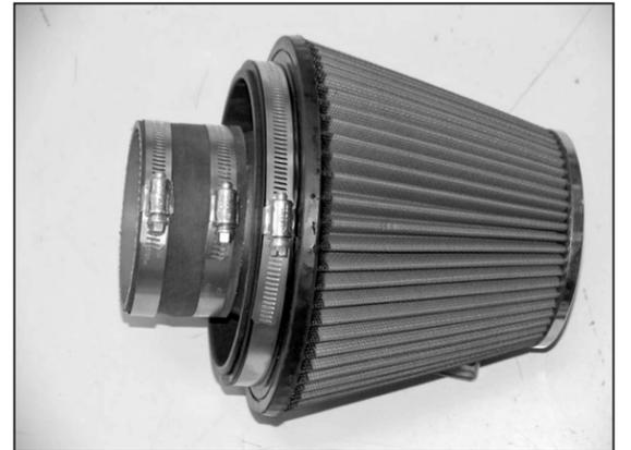
26. Install the silicone hose (08630) onto the Air filter adapter as shown and secure with the provided hose clamp as shown.
