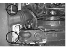
11. On vehicle's equipped with an air box cover, remove the two bolts which secure the cover to the frame rail, and the bolt which secures the intake snorkel to the radiator core support.
