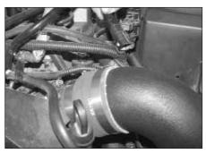
27. Reconnect the crank case vent hose to the fitting installed into the K&N intake tube in step #16.
