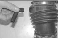
16. Remove the crank case vent fitting from the factory intake tube as shown.
