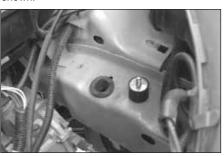
25. Install the rubber mounted stud into the threaded hole in the frame rail as shown.
