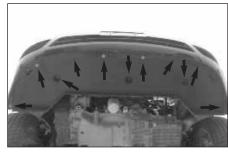
10a. On vehicle's equipped with the splash shield, remove the six bolts and five plastic screws which secure the splash shield to the bumper cover, then remove the splash shield from the vehicle.
