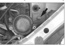
8. Remove the bolt, which secures the mass air sensor housing bracket to the inner fender.
