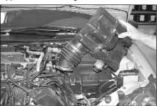
5. Lift firmly to separate the upper intake housing from the mass air sensor housing and then remove the upper intake housing from the vehicle.
