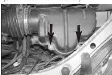
Loosen the two bolts, which secure the upper intake housing to the mass air sensor housing.
