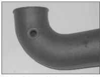
17. Install the provided grommet into the K&N intake tube as shown.
