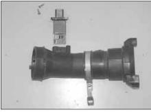
19. Remove the mass air sensor from the factory mass air sensor housing using the Torx wrench
