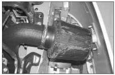
29. Install the air filter onto the K&N intake tube and secure with the provide hose clamp.
