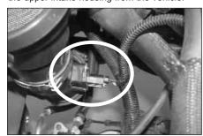
6. Depress the locking tab on the mass air sensor electrical connection and then disconnect the electrical connection.
