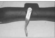
24. Install the provided bracket (010063) onto the K&N intake tube with the provided hardware as shown.
