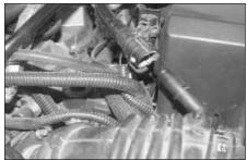
2. Depress the green locking tab on the crank case vent hose and then pull the vent hose to disconnect from the fitting as shown.
