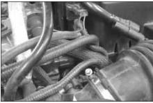
3. Loosen the hose clamp, which secures the factory intake tube to the throttle body.
