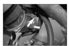
7. Loosen the hose clamp, which secures the mass air sensor housing to the lower intake housing.
