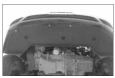
30a. On vehicle's that were equipped with the splash shield, reinstall with the bolts removed in step #10.
