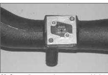
23. Secure the mass air sensor assembly into the K&N intake with the provided hardware as shown.
