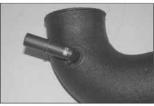
18. Install the crank case vent fitting removed in step #16 into the grommet installed into the K&N intake tube in step #17 as shown.
