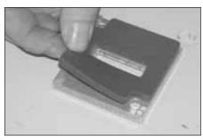
20. Apply the provided gasket onto the K&N mass air adapter as shown.
