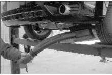
14a. On vehicle's equipped with the upper intake snorkel, pull down on the snorkel to dislodge it from the mount and then remove it from behind the fender.
