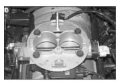
16. Install the tube mounting bracket assembly onto the throttle body and secure with the factory bolts removed in step #14. Torque the throttle body bolts to 17ftlbs.
