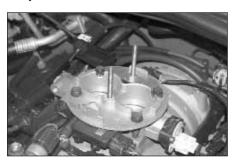
17. Install the provided stud into the threaded hole on the throttle body and tighten completely. NOTE: Apply two drops of thread locker to the stud and torque to 30 inch pounds. Failure to follow the above instructions may damage the throttle body.
