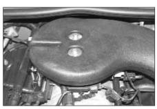
21. Secure the intake tube with the provided nut and washers as shown.
