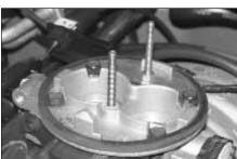
18. Install the provided gasket onto the throttle body sticky side down.
