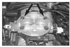
14. Remove the two rear throttle body bolts as shown.
