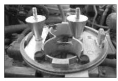
19. Install the provided stand off's onto the studs as shown.
