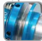
Springs twist during extension and compression. The King 3 Piece coil nut allows the springs natural rotation without binding.
