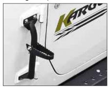
Foot pegs mount to JK door hinge assembly, front or rear, about 15" above Rocker Walk. Provides a mid-step solution between Rocker Walks, Kat-Walk and JK roof top. Permits easy access to cargo on the roof. Ideal use with: Rocker Walks and Kat-Walk. Sold in pairs.
