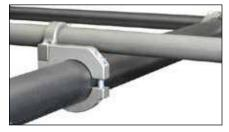
Multi-purpose mounting solution. Adjustable Hard anodized, machined billet aluminum brackets for intersect or parallel attachment of 1-1/8" dia. Aluminum load bars or other aftermarket load bars to cage rails. Sold in pairs.
