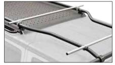
60" hard anodized aluminum universal load bar, lightweight and strong, 1-1/8" standard diameter. Permits attachment of recreational equipment and cargo carrying products. Use with KM Safari specialty brackets and clamps for greater versatility and load configuration options including Cross Over Clamps or Standoff Brackets. Easily cut to any length.
