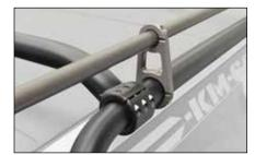
A great way to attach a load bar to a Congo Cage. Hard anodized and machined billet aluminum brackets. Opposite side of bracket has a 1-1/8" mounting hole for aluminum load bar (#60335) or other aftermarket load bars. Can be used on "Classic" Congo Cage tube diameter. Parallel design with 4" offset, not cross over. Sold in pairs.
