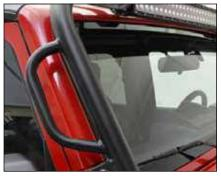
The Front Hoop for the JK Congo Pro #55000 & #55010 has a built-in Grab Handle on both sides which aids one in accessing the Jeep roof or optional Kat-Walk. Available without handle #55016.
