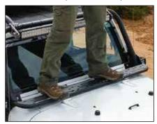
Mounts on JK Front Hoop as a non-slip step platform, spans windshield/hood area of JK. Bolt-on use with JK Front Hoop. Made of high grade tubular steel, supports 350 lbs.
