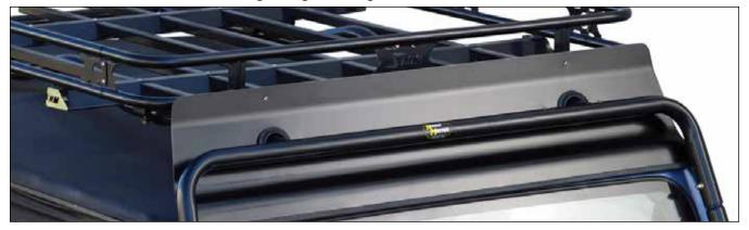
KM Safari racks are designed to minimize wind noise, but sometimes basket location, cab lights, atmospheric conditions or other accessories can cause noise. This wind deflector bolts to the front cross bar, and can be positioned to optimally deflect wind up over the cab, reducing or eliminating noise.
