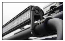
The trickest light mounts money can buy. CNC machined and hard anodized billet aluminum clamps. Mount aftermarket light bars to any 2" KM Safari product, including: Front Hoop, Roof Rails and Rear Hoop. Max light bar length 42" on Front Hoop. Light bar not included.
