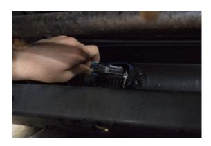
**9.** When the existing and new fog light horizon lines are aligned, use the 4 existing mounting screws to install the lamp assembly to the bumper.
