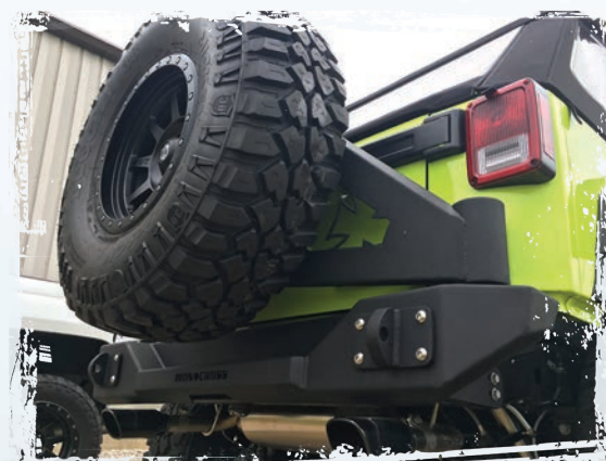
Heavy Duty Swing Away Tire Carrier Accommodates up to a 42" Tire
