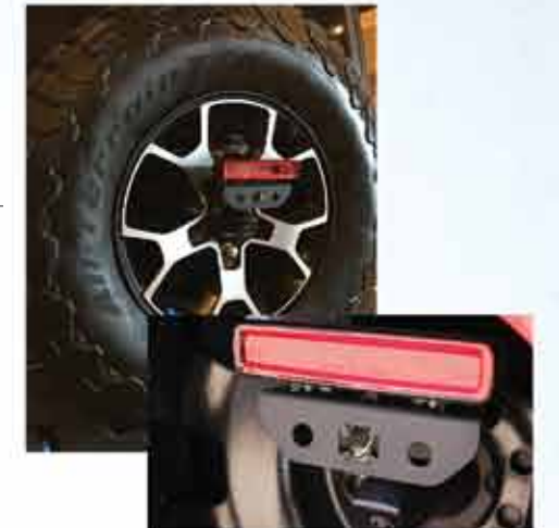
#GP-0400 - Jeep JL 3rd Brake Light & Backup Camera Relocation Bracket
