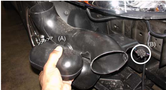
With the front bumper out of the way (A), remove the plastic clip (B) that secures the stock resonator duct in the front bumper passenger area. Continue to remove the air resonator duct in order to make room for the Injen filter.
