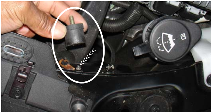
Take the male/female vibra-mount in this kit and screw the female end over the threaded stud securing the grounding wire..
