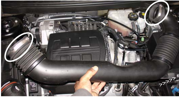
Loosen the clamps and m6 bolt to remove the stock air intake duct that connects the stock air box to the throttle body.
