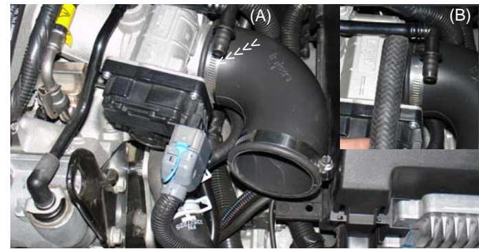
Press the 2 3/4" silicone elbow over the throttle body. Use two clamps in this kit to place them over the ends of the silicone elbow, semi-tighten the clamp on the throttle body side. Take the 12mm hose and press one end over the crankcase hard pipe as shown in the picture (B).
