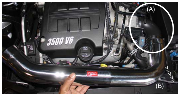
Take the primary intake and press the end with the 90 degree bend into the elbow on the throttle body (A). Once the intake has been pressed into the silicone, align the bracket on the intake to the vibra-mount stud (B).
