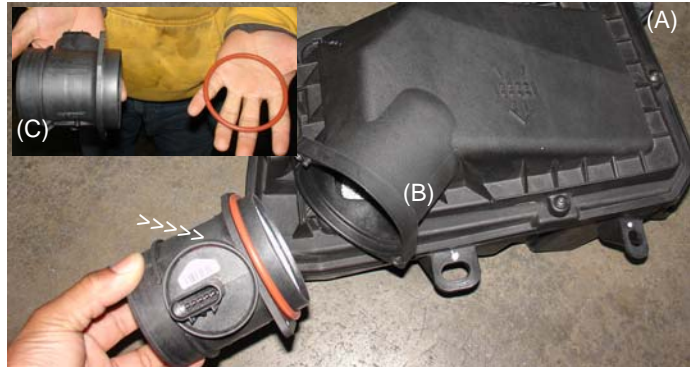
Loosen the m6 bolts that secure the stock air box to the mounting points. Remove the air intake box from the engine compartment (A). Once the stock air box has been removed the engine compartment loosen the bolts that hold the mass air flow sensor to the stock air box (B). Remove the O-ring from the mass air flow sensor which will not be used in this installation (C).
