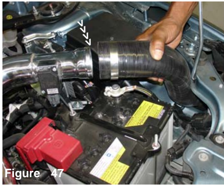
Figure 47 Once you have lower the lower end into the resonator opening, continue to align the intake to the primary aluminum intake.
