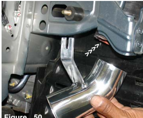
Figure 50 Align the extended intake to the secondary silicone hose as shown above.
