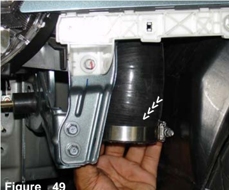
Figure 49 Slip one power-band over the end of the secondary silicone.
