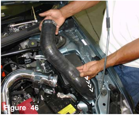
Figure 46 The secondary silicone hose is now lowered into the engine compartment.
