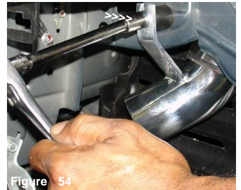
Figure 54 The 8mm socket is used to tighten the m6 flange nut over the vibra-mount stud.
