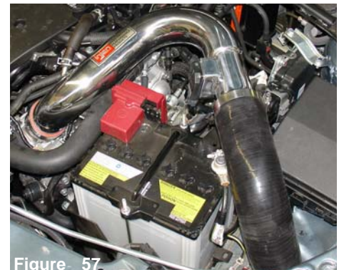
Figure 57 Congratulations! you have just completed the installation of this intake system. Periodically, check the fitment of the intake system for misalignment that may occur over time.
