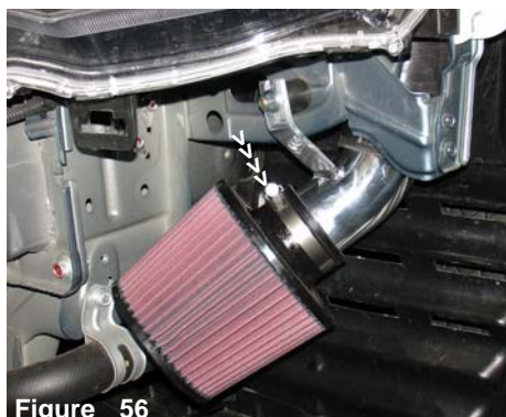
Figure 56 Once the intake end has butted up against the filter stops, continue to tighten the filter neck clamp.
