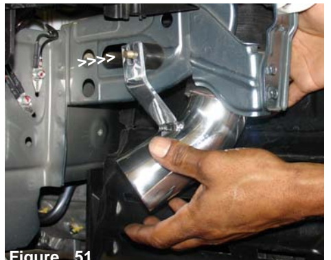
Figure 51 Press the extended intake to the secondary silicone hose and align the intake bracket to the vibra-mount stud.
