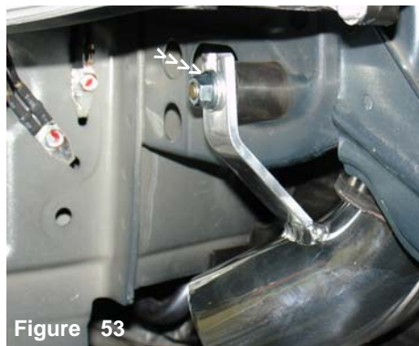
Figure 53 Use the m6 flange nut and fender washer to fasten the intake bracket to the vibra-mount stud.
