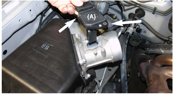
Remove the screws from the mass air flow sensor (A) and carefully pull the air sensor out of the sensor housing.
