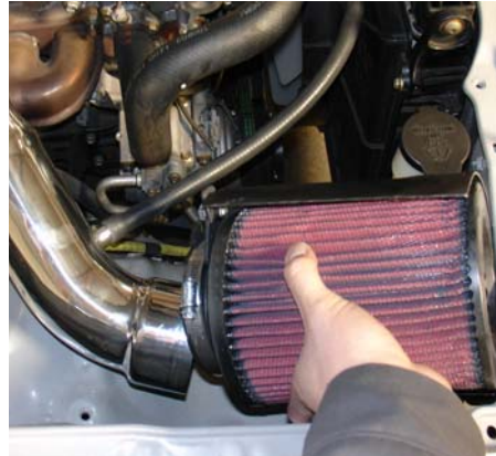
The 3 1/2" inverted top filter is set in the engine compartment ready to be installed.
