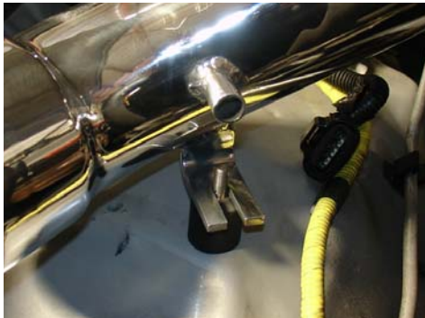
The intake bracket is sitting flush over the vibra-mount stud and lined up to the throttle body.
