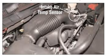
Route the Interceptor wire to vehicle intake air temp sensor.
