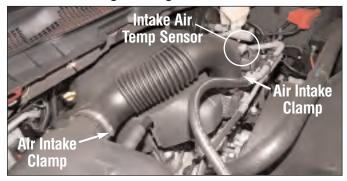
To access the MAP sensor, you must remove the air inlet tube. First, disconnect the intake air temp sensor, and then loosen the clamp at the throttle body using a flathead screwdriver.
