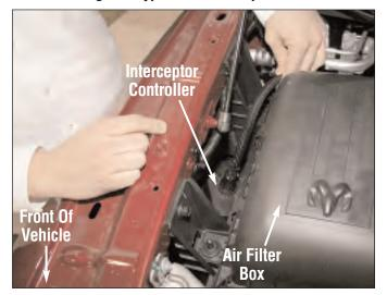
Position and mount the Interceptor Controller on the passenger side of the vehicle as shown between the fenderwell and the air filter box. Use the provided velcro to secure it to the vehicle.
