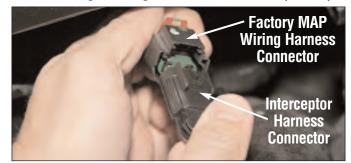
Plug the Interceptor harness connector into the factory MAP wiring harness connector, and push in the locking clip. Reinstall the engine beauty cover then the intake hose removed in the previous steps. *DO NOT reconnect the air intake sensor as it will be reconnected in the next section of the Interceptor installation.*
