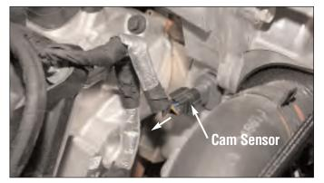
Route the Interceptor wire to the cam sensor. Disconnect the factory harness from the cam sensor.
