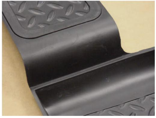
TRIM ALONG INTERSECTION OF THE "STEP" IN THE PART AND THE PORTION OF THE LINER THAT CONTINUES OVER THE HUMP. THIS WILL LEAVE A "LIP" ON THE TRIMMED LINER AS SHOWN IN THE PHOTO BELOW.
