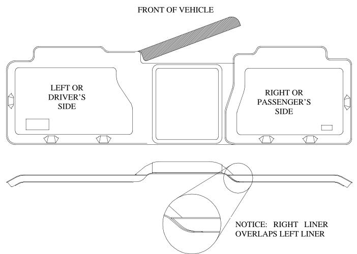
YUKON DENALI OWNERS WILL NEED TO TRIM THEIR LINER TO ACCOMMODATE THE FACTORY EQUIPPED CONSOLE. TRIM AWAY THE MATERIAL ON THE LINER THAT IS LOWERED AS DEMONSTRATED ABOVE AND AS SHOWN ON THE PHOTOS ON THE REVERSE SIDE.
