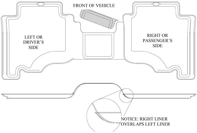
GRAND CHEROKEE OWNERS WHOSE VEHICLE ARE EQUIPPED WITH THE FACTORY DVD PLAYER (ELECTRONIC INFOTAINMENT SYSTEM) WILL NEED TO TRIM THE CENTER HUMP PORTION OF THEIR DRIVER'S SIDE LINER TO ACCOMMODATE THIS OPTION. TRIM YOUR LINER AS SHOWN ABOVE USING THE MOLDED IN GROOVE AS A GUIDE (SEE PHOTOS ON BACK). A UTILITY KNIFE OR SCISSORS WORK WELL FOR TRIMMING.
