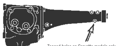
CHEVROLET (341) 4-bolt side cover with round-gear selection shafts Tapped holes on Corvette models only
