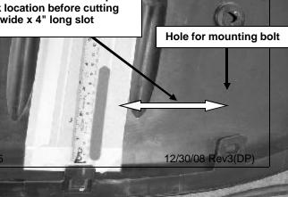
Cut only what is needed to insert bracket through the splash guard. Do not cut through the front edge of the splash guard
