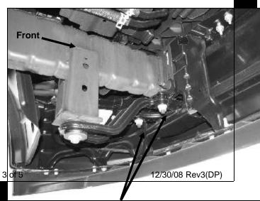
(Fig 2A) Driver side mounting locations viewed from behind the bumper (non tow hook equipped models)
