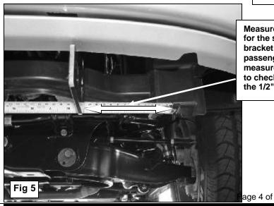
Measure from the mounting point for the splash guard to the bracket on the driver and passenger sides. Use this measurement as a reference point to check location before cutting the 1/2" wide x 4" long slot
