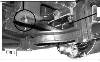
Hold the splash guard up to the brackets and mark location for cutting to clear brackets. Cut only what is needed to insert bracket through the splash guard.
