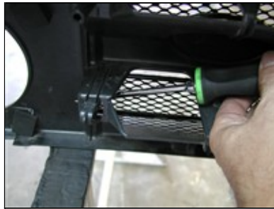
Picture #8: UPPER GRILLE INSTALL.
