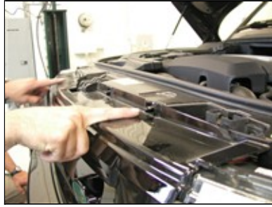
Picture #2: UPPER GRILLE INSTALL.
