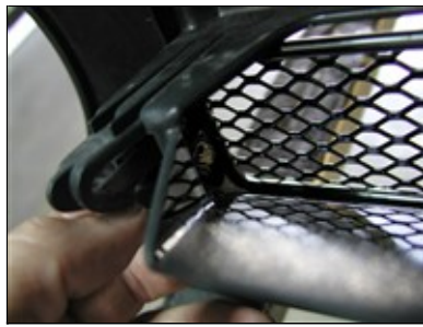
Picture #35: LOWER GRILLE INSTALL
