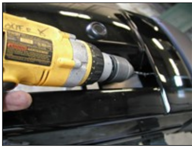
Picture #34: LOWER GRILLE INSTALL
