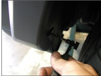
Picture #20: LOWER GRILLE INSTALL
