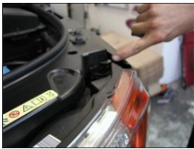
Picture #16: LOWER GRILLE INSTALL
