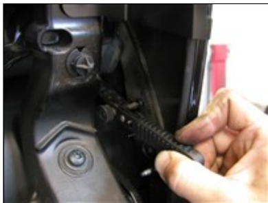
Picture #22: LOWER GRILLE INSTALL
