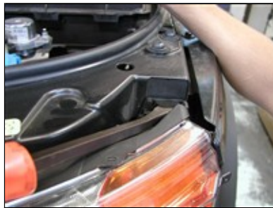
Picture #14: LOWER GRILLE INSTALL
