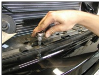
Picture #26: LOWER GRILLE INSTALL
