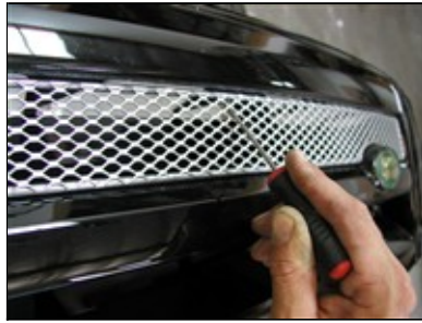
Picture #5: UPPER GRILLE INSTALL.
