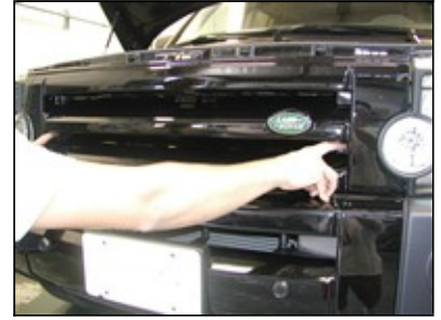
Picture #3: UPPER GRILLE INSTALL.
