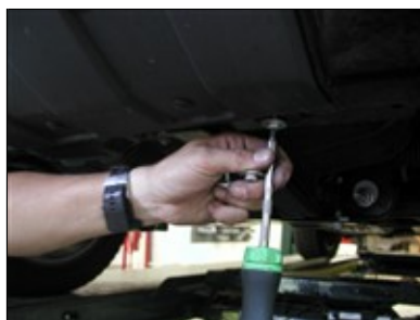
Picture #29: LOWER GRILLE INSTALL
