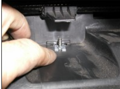
Picture #37: LOWER GRILLE INSTALL
