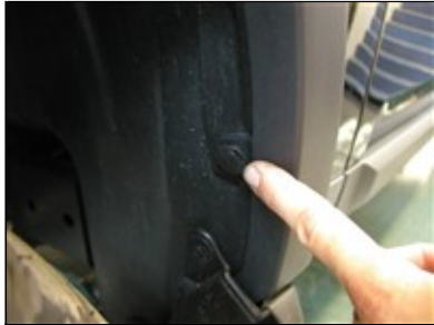
Picture #19: LOWER GRILLE INSTALL
