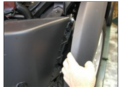
Picture #24: LOWER GRILLE INSTALL
