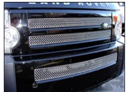
Picture #45: LOWER GRILLE INSTALL FINISHED!
