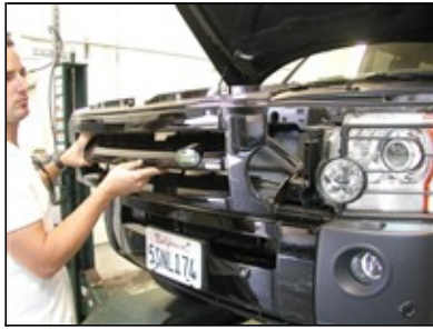
Picture #4: UPPER GRILLE INSTALL.
