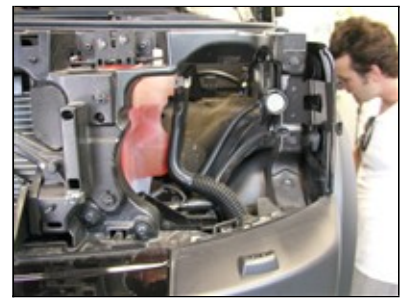
Picture #18: LOWER GRILLE INSTALL
