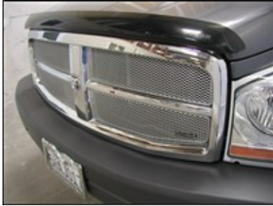
Picture #16: Done!!! Dodge Durango Custom Grille installation.
