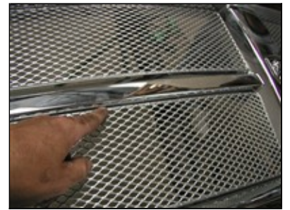
Picture #15: Position the grille in order to leave the gap on the bottom of each insert.
