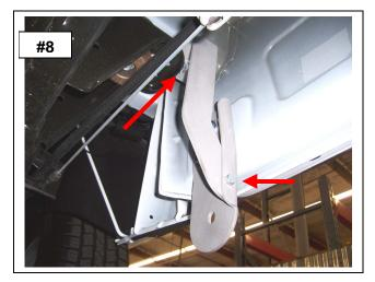
**STEP-9** ATTACH THE DRIVER SIDE STEP TO THE FRONT AND REAR BRACKETS USING (1) 1/2" X 2" HEX BOLT, (1) ½" FLAT WASHER AND (1) 1/2" LOCK WASHER FOR EACH BRACKET.
