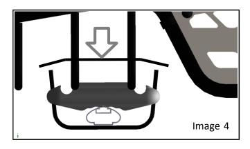
5. Secure each thread of the "U"-bolt with a Knob nut.
