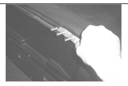
Step 3. Slide the bolt plates into rail tracks and position them toward the front of the bed.
