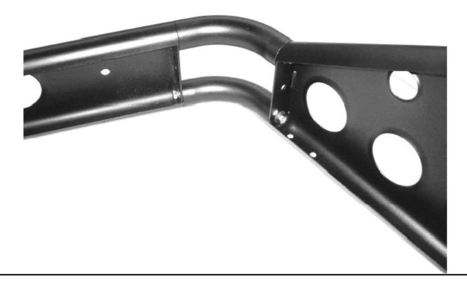
Step 7. Secure the sport rack assembly nuts and bolts.
