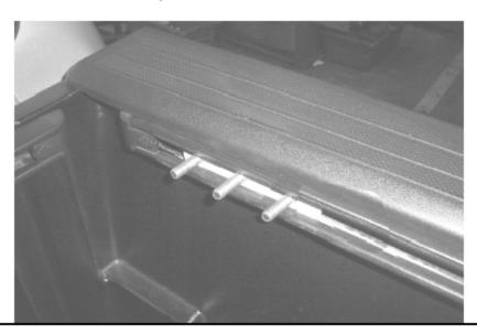
Step 4. Secure the rail tracks and reinstall the tie downs and rail end plugs
