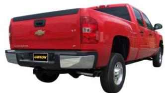
8. Install stainless steel tip. Clamp down. When you have everything in place, firmly tighten all bolts and clamps down securely. Use stainless steel cleaner and a Scotch Brite pad weekly to prevent tip from discoloration. Inspect all fasteners after 25-50 miles of operation and re-tighten as necessary.
