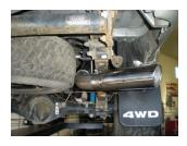
8) Place the ST429 stainless tip onto the end of the tailpipe and adjust to the desired location. Tighten the nut on the clamp to secure the tip in place.
