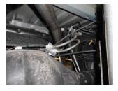
Place left front tailpipe section **#26430S** into position over the rear axle and slide into the left muffler outlet. Place a supplied 3" clamp onto the back of the pipe. Place left rear tailpipe section **#26432S** onto the front section, and connect the hanger welded to the rear of the pipe into the rubber hanger installed in step 3 above. Pipe should be centered between the shock and the spare tire when adjusted. Tighten the clamps just enough to hold in position.
