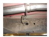
2) On Crew Cab - 5.5" bed model trucks, slide hanger assembly **#481HA** over the back of the inlet pipe and connect to the rubber mount on the vehicle. On Extended Cab - 6.5" models do the same with hanger **#480HA**. Tighten the ring clamp enough to hold, but still allow for adjustment.
