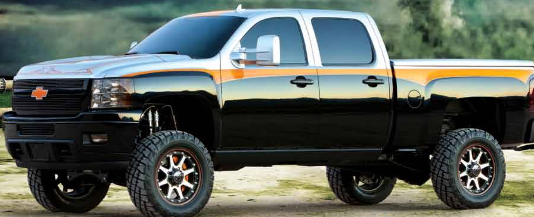
2011 GM K2500HD W/ 35" TIRES • 6" RTSM™ SYSTEM • 35/13.50R20 TIRES • 20X10 WHEELS W/ 5 3/4" BACK SPACING
