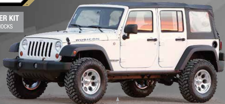
3" SPACER KIT - PERFORMANCE SHOCKS 35/12.50R17 TIRE W/ 17X9 WHEELS W/ 5" BS
