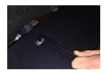
Install the 3/8" hex cap bolt with corresponding washers and nyloc (again using washers on both the nut and bolt sides), in the holes previously drilled out. Again keep all nuts and bolts loose until the end.
