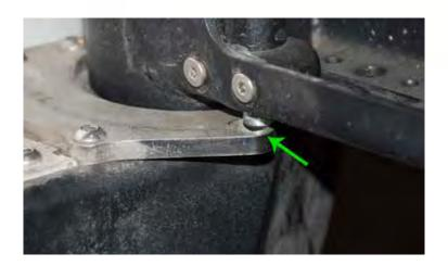
Adjust the button head bolts as shown until the pin drops into place. Then secure down again.
