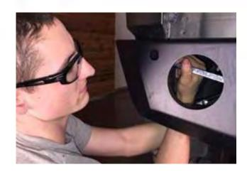
In the center step of the bumper there are 2 holes for 1/2" button head bolts. These bolt locations are mainly used for the optional winch mount and are not required for regular use; however, if you desire to install the bolts we recommend using the additional USS flat washers a shims between the bumper and the factory receiver hitch assembly.
