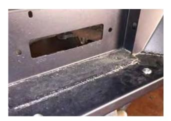
Lay your spare tire on the ground and set the tire mount into place. Now set the arm on top of it, marking the height when the arm is flat across it.
